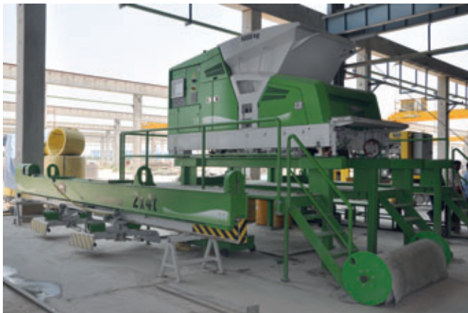
Extruder E9 and lifting beam
