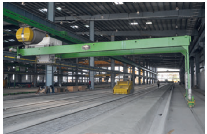
Hollow-core casting line with automated concrete distribution
