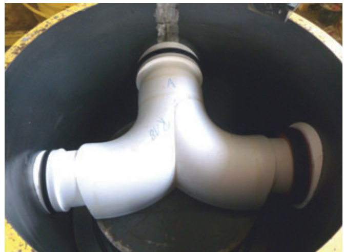
The mounting of the formwork – in an ideal manner including preassembled seals – depicts the final preparation step of exact negative channels
