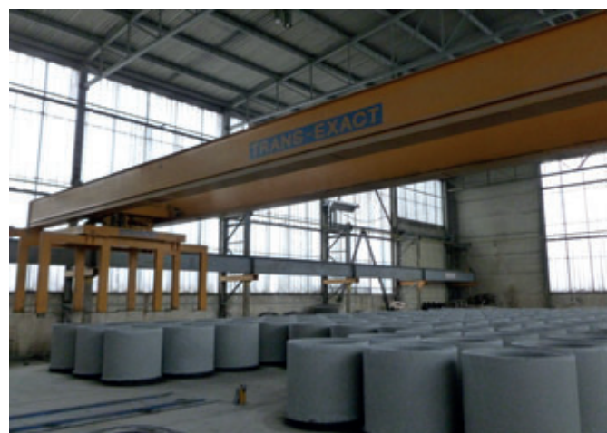
A crane robot is a central component of highly-automated manhole ring and cone production installed at the beginning of the 1990s
