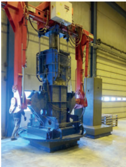
Demoulding at the curing station
