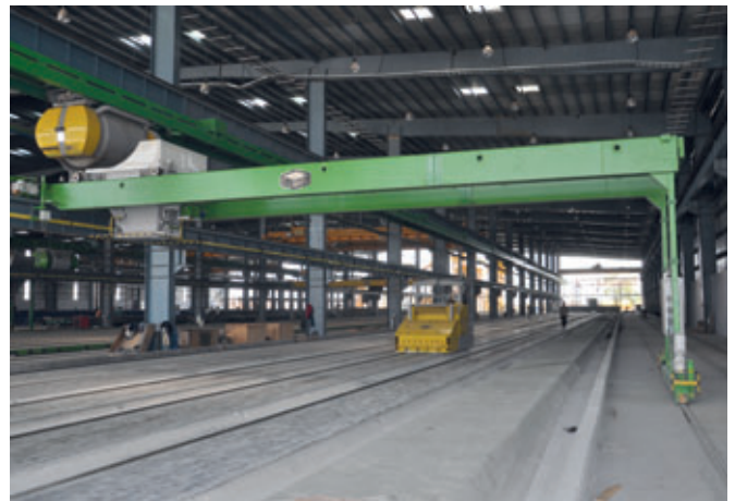
Hollow-core casting line with automated concrete distribution
