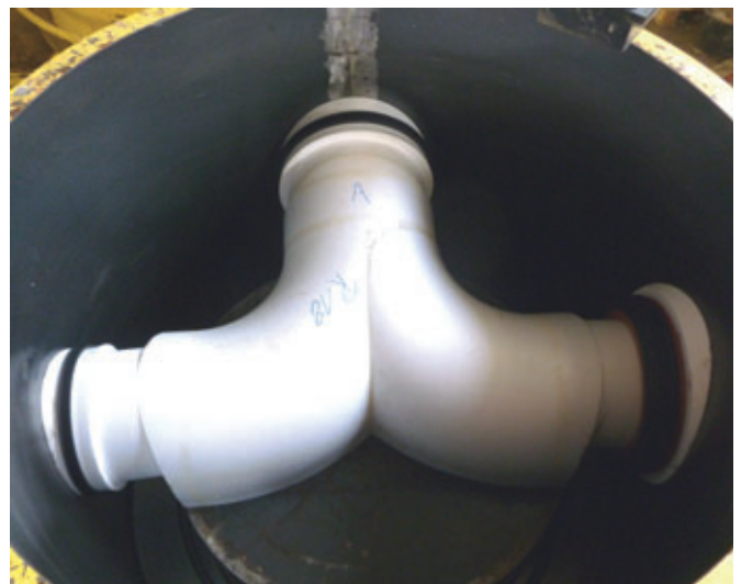
The mounting of the formwork – in an ideal manner including preassembled seals – depicts the final preparation step of exact negative channels
