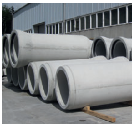
At Grafe Beton, wet-cast concrete pipes are manufactured for open construction up to a nominal width of DN1200
