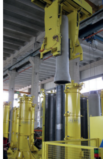
After curing in the formwork, the jacking pipes are demoulded the following working day
