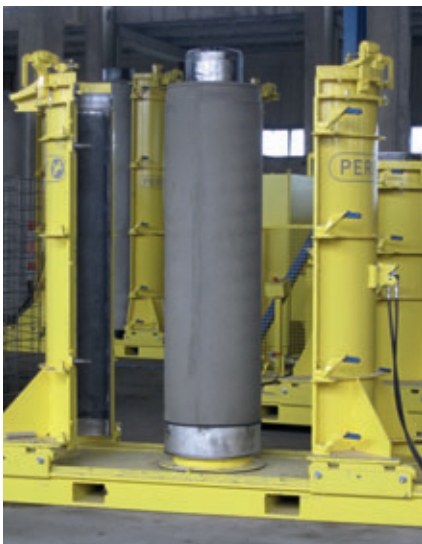
For future projects, the Perfect Pipe jacking pipes are produced to a nominal width of DN300 in 2 m lengths
