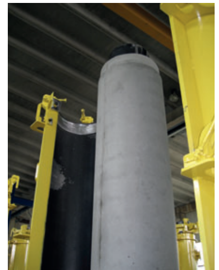
Concrete pipes made using liquid concrete are wet-cast and therefore manufactured to exceptionally low tolerances
