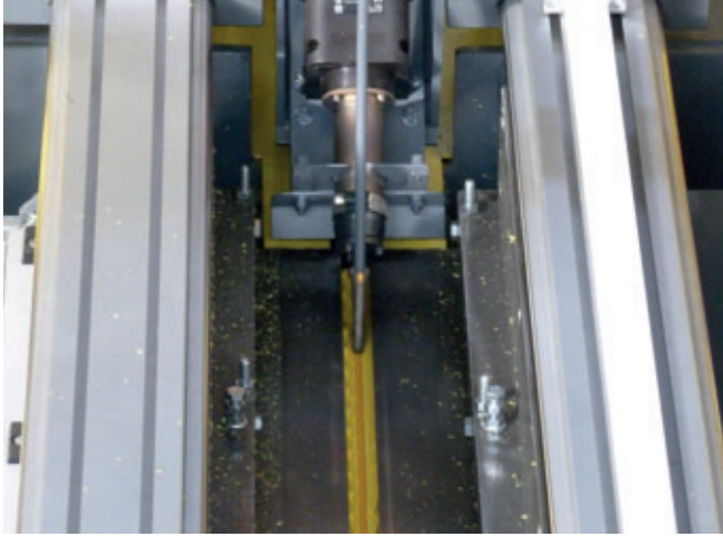
The HDPE liner is welded to a tight pipe liner
