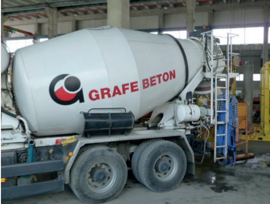
The concrete is mixed using trucks to produce jacking pipes and poured into the moulds using a pail
