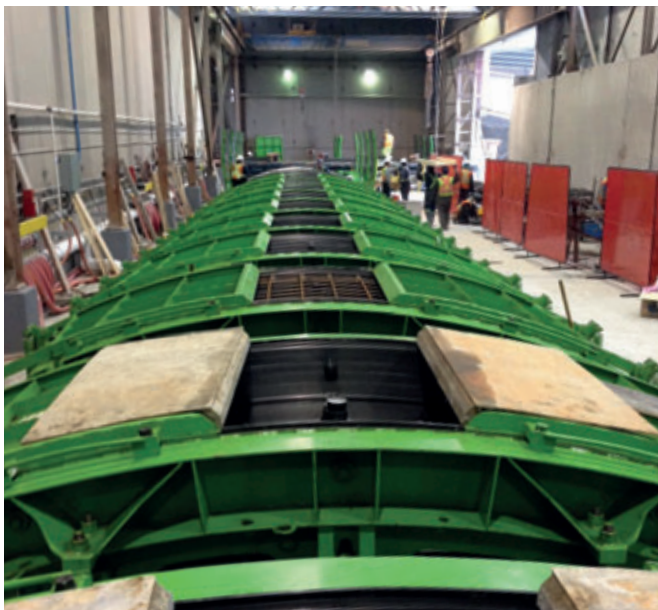
Evergreen Mold Segments cleaned and ready to pour concrete, molds are poured twice a day producing 48 segments a day which equals 6 tunnel rings.
