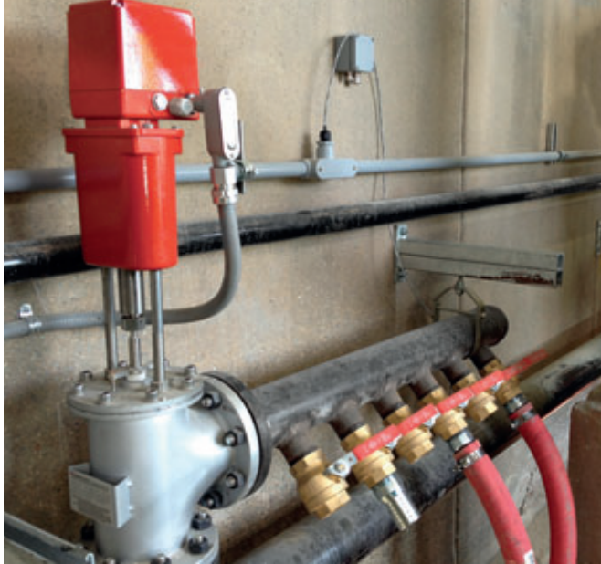
Vapor control valve with hose connections to inject vapor underneath the molds.
