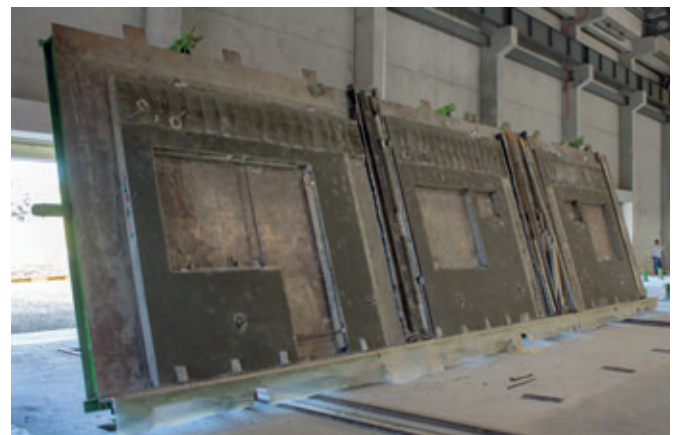
Precast facade panels at tilting station
