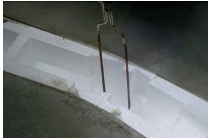
The intelligent design of the preformed parts simplifies the demoulding process and reduces the volume of recycling material
