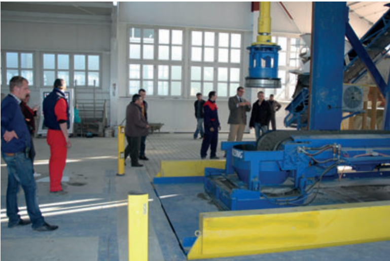
Production of pipes during the official presentation of the Prinzing Tornado
