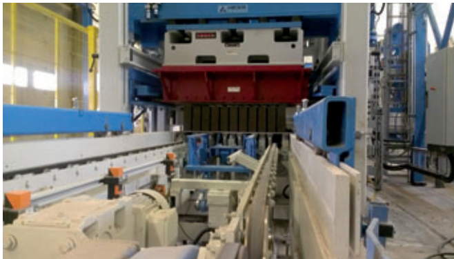
Hess RH 1000-2 high-performance machine with electric mould change carriage
