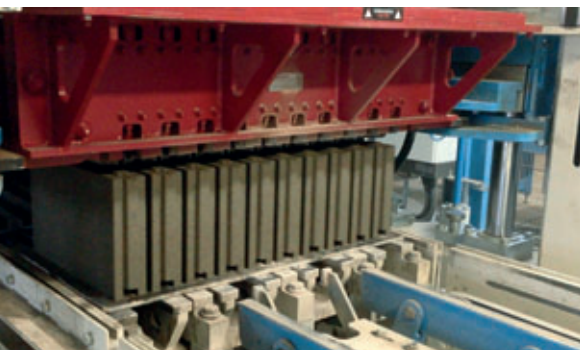
Complex blocks with a horizontal and vertical tongue and groove system
