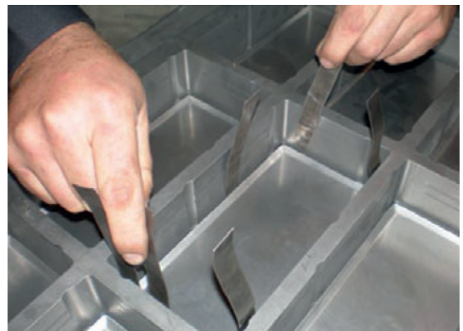
Pressure plate replacement
