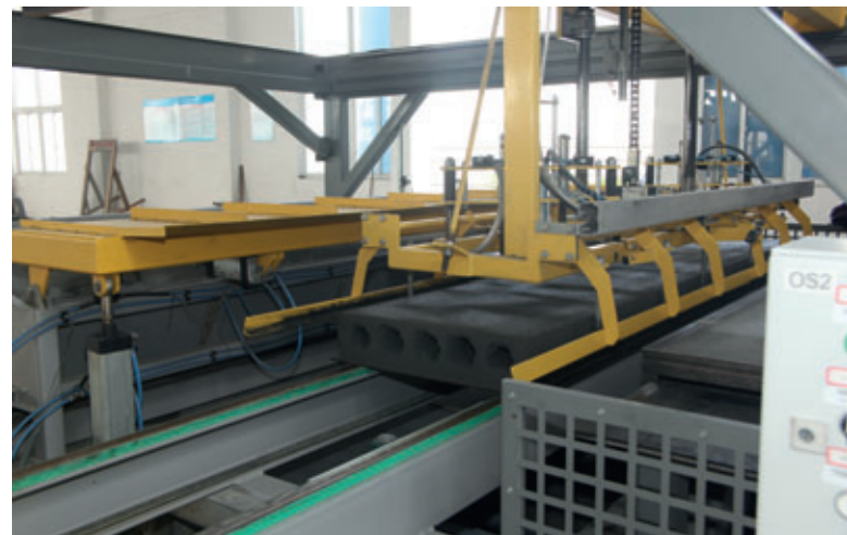
At the Stacking station of the Acotec line the fresh panels with the base plate are stacked in 6-10 panel stacks for curing.
