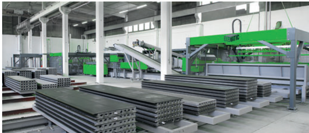
Fresh Acotec Panel stacks on their way to the overnight curing storage.
