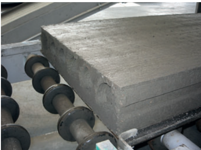
Fresh cut Acotec panel on its way to stacking.
