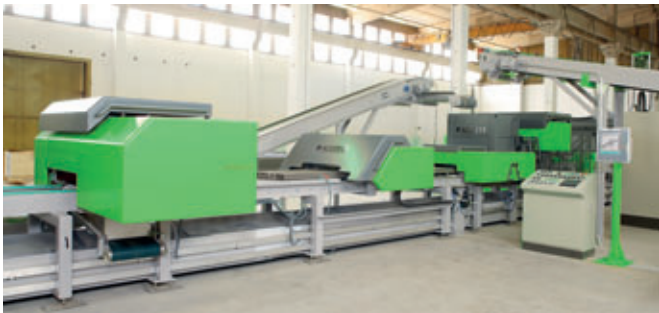
The heart of an Acotec line is made of a stationary extruder and a saw that cuts the products on fly.
