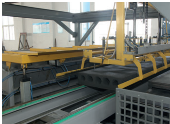
At the Stacking station of the Acotec line the fresh panels with the base plate are stacked in 6-10 panel stacks for pre-curing.
