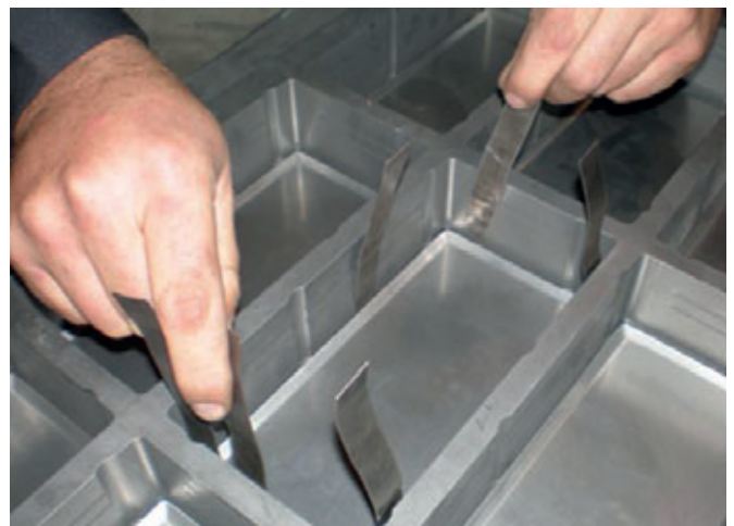
Pressure plate replacement
