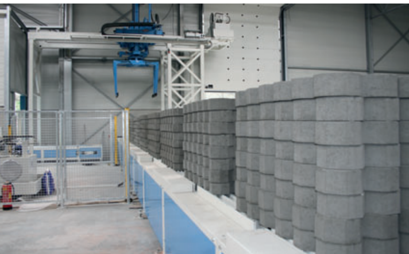
The walking beam conveyor transports the block packages to the package transfer device
