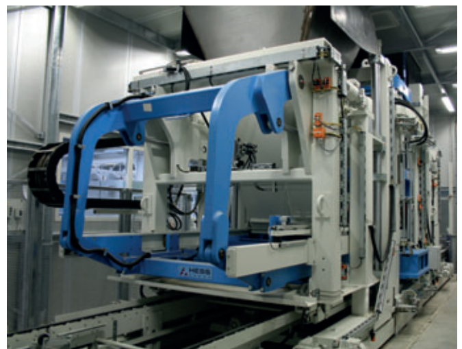
All components that are subject to stress are of a particularly sturdy design in the Multimat from Hess
