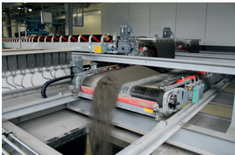
The belt conveyors from VHV Anlagenbau transport the concrete from the mixers to the concrete block making machine
