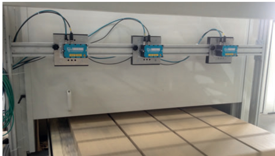
The SHV 500 block height measuring system from R&W Industrieautomation monitors the height accuracy of the fresh products.
