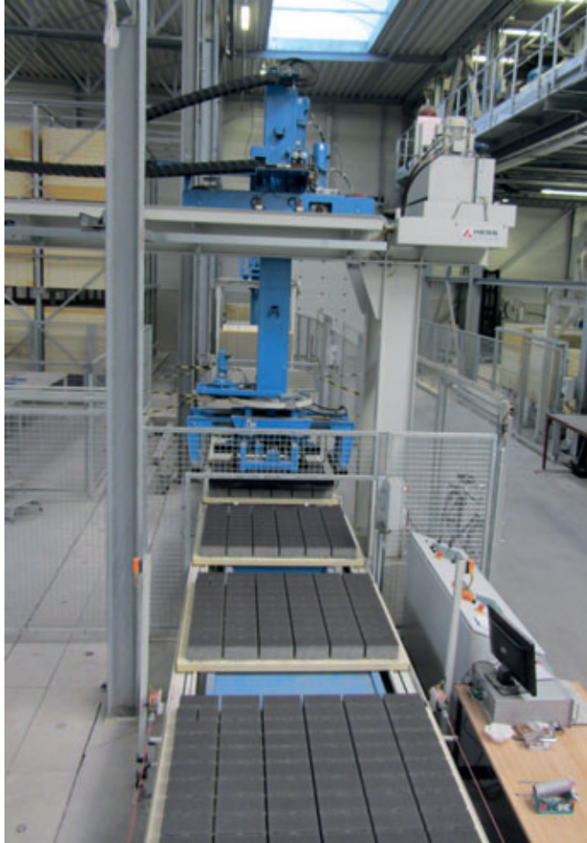
Dry side with Servo 700 packet assembler
