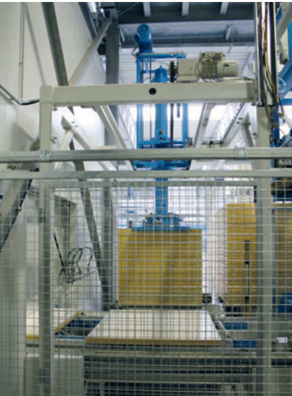
The transfer device places the production boards of a package on the board intake of the block making machine
