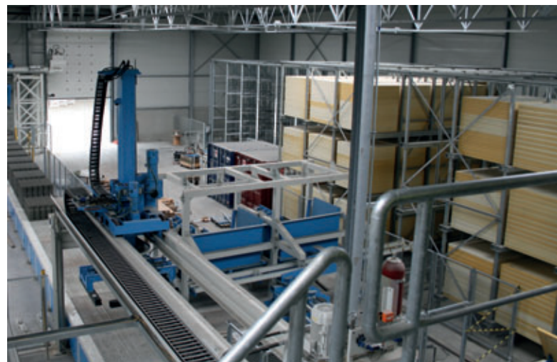
Servo 700 packet assembler from Hess on the dry side, mould rack and board buffer rack
