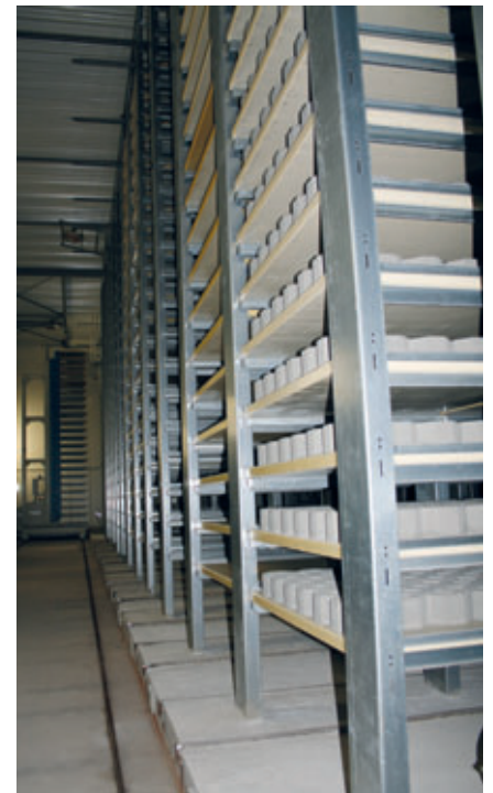
The curing rack from Rotho offers space for up to 6,776 production boards
