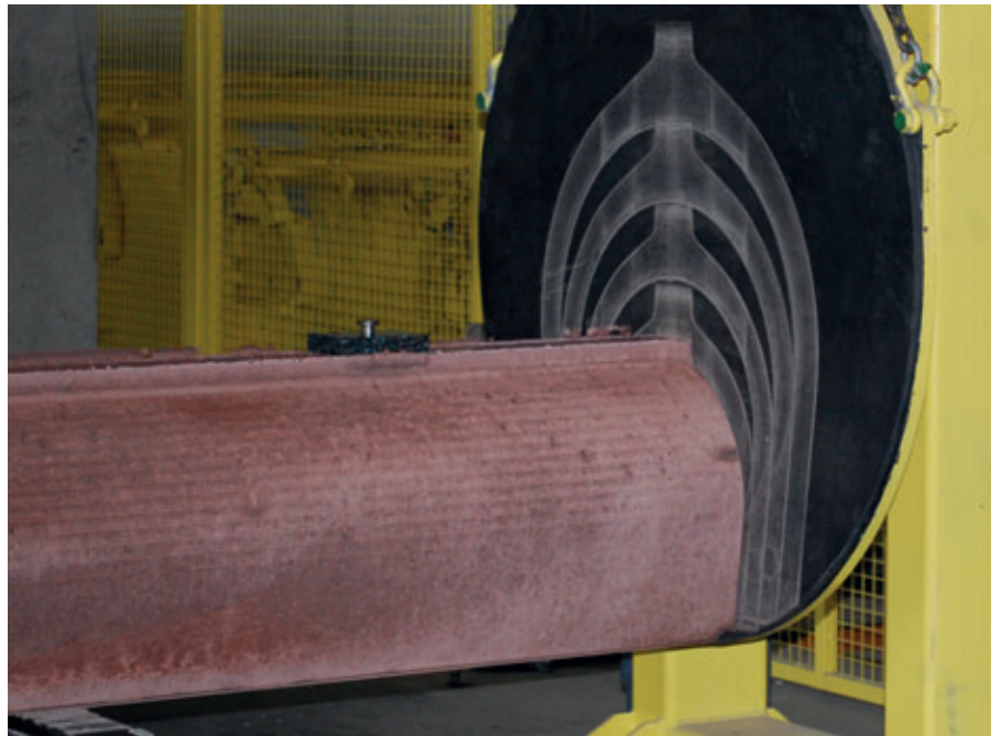
The wet-cast pipe made of self compacting concrete is subjected to a leak test in fully automated production before final approval.
