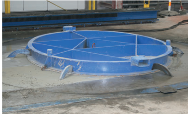
The container is made absolutely watertight by pressing and compacting again.
