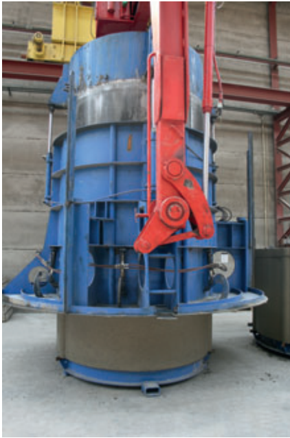
The complete demoulding process is controlled from the pendant crane control.
