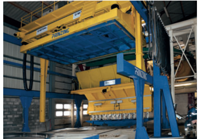
Zelus plant from Prinzing with concrete feeding and crane robot
