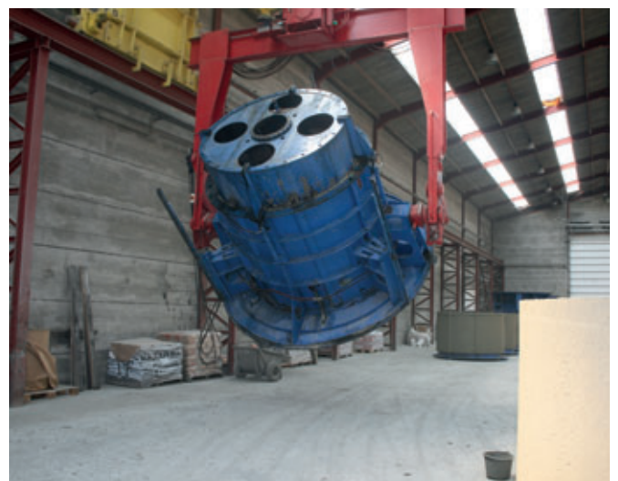
The mould is hydraulically turned during transport to the demoulding station.
