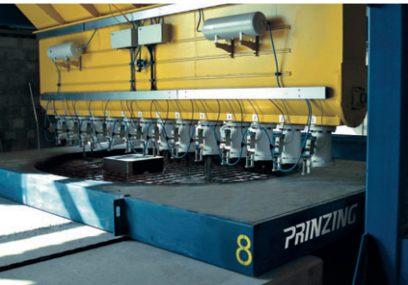
The fully automatic Zelus casting plant fills the mould with self-compacting concrete via individually controlled pinch valves
