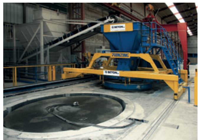
Production takes place on production station 1; the concrete silo is filled in the central position and production station 2 is prepared for the next product.
