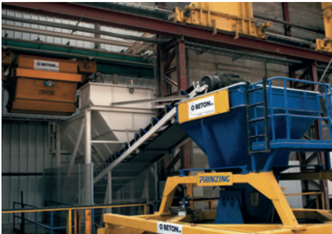
The Atlas is supplied with earth-moist concrete via a bucket track and a pre-silo
