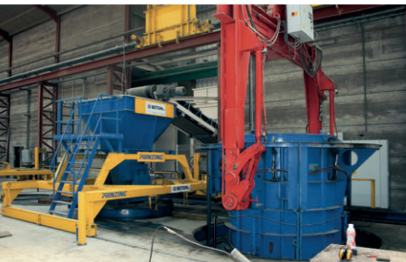
During the removal of the mould the material silo at the central position is filled again.
