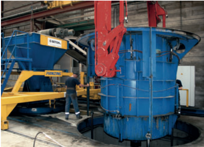
After demoulding the mould is put back into the workstation and the next product can be manufactured.
