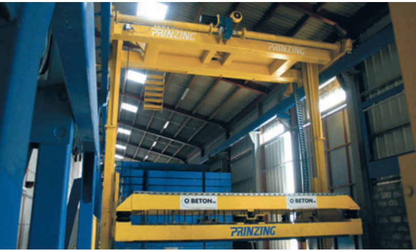
A crane robot fully automatically manages and operates the mould store of the Zelus casting plant.
