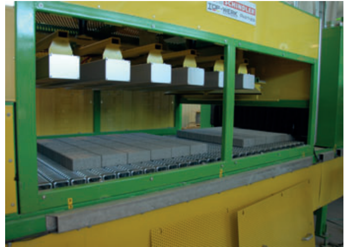
Infrared heating tunnel with six heaters
