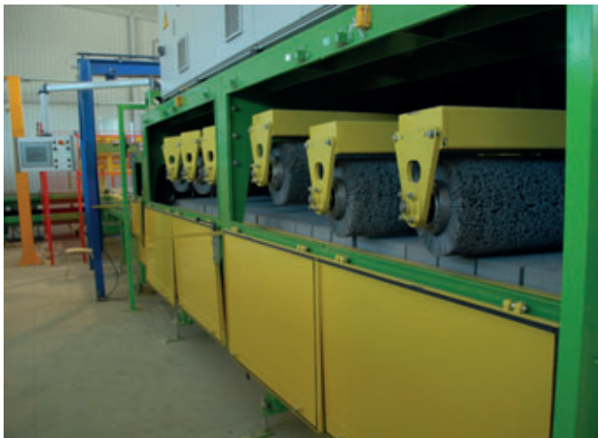
Curling machine with six brush rollers
