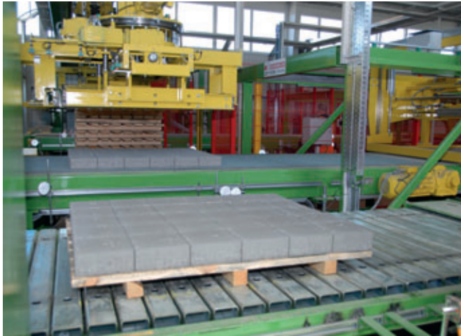
Four-sided clamp for inserting the stone layers into the finishing line; the pallet buffer can be seen in the background
