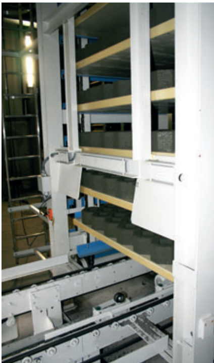
The elevator can accept up to 22 production boards
