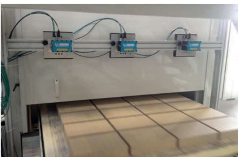
The SHV 500 block height measuring system from R&W Industrie-automation monitors the height accuracy of the fresh products.
