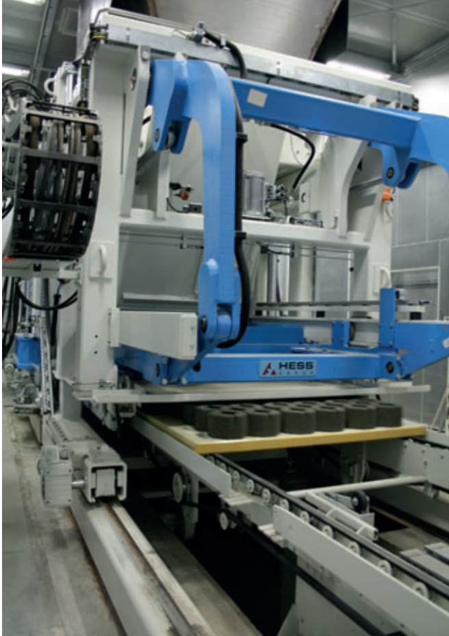
The production boards with the fresh products are transported to the hardening chamber by the V-belt conveyor.
