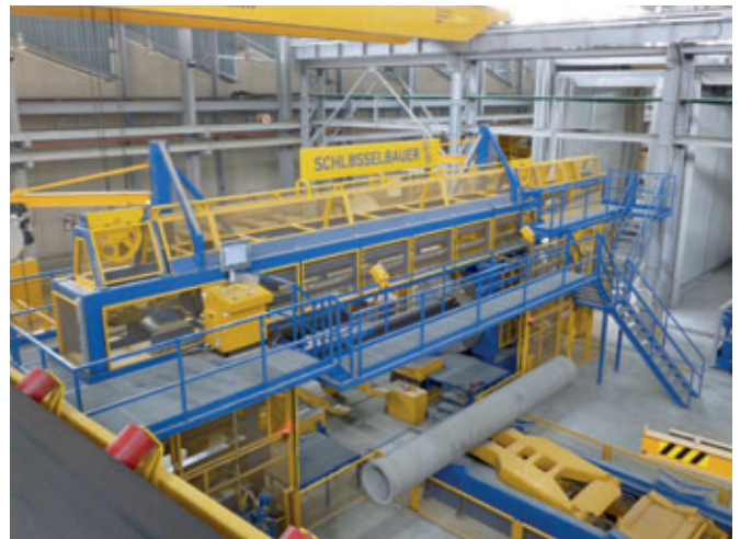
The speed and precision of wire pre-tensioning for pressure pipe production were increased by Schlüsselbauer's current new developments.
