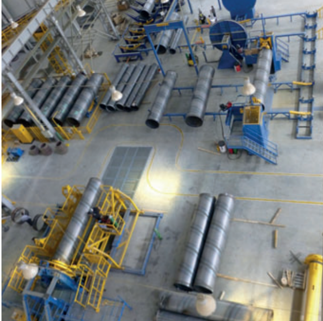
The manufacture of steel cylinders under controlled conditions is a central element of concrete pressure pipe production.
