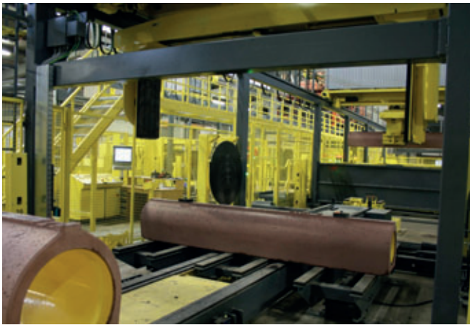
Before exiting the production line, each pipe is tested for leaks.
