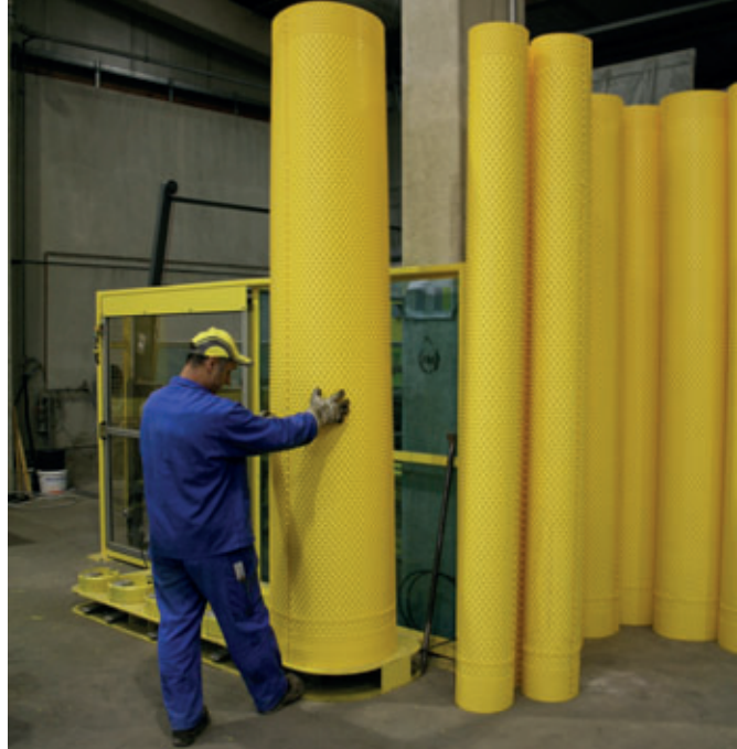
The tensile strength of the welded seam can be checked immediately after the welding process is complete.
