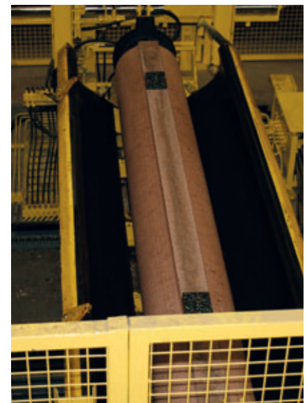
Demoulding a cured Perfect Pipe
