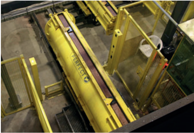
A full mould leaves the concrete pouring station.
