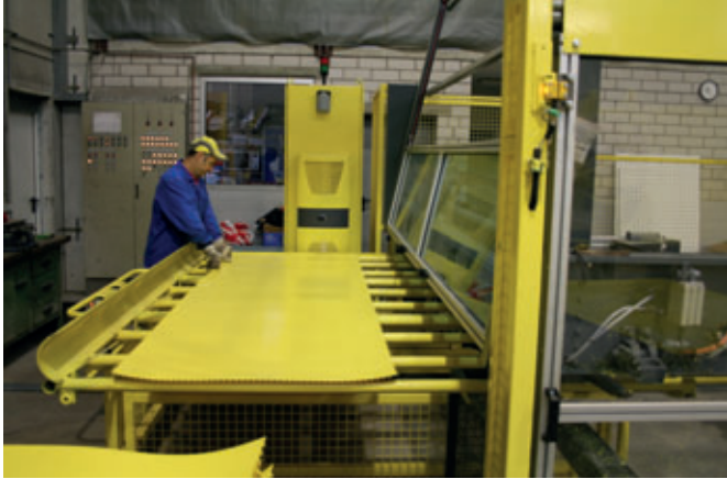
The PE film is precisely cut to length and is then pushed into the welding machine.
