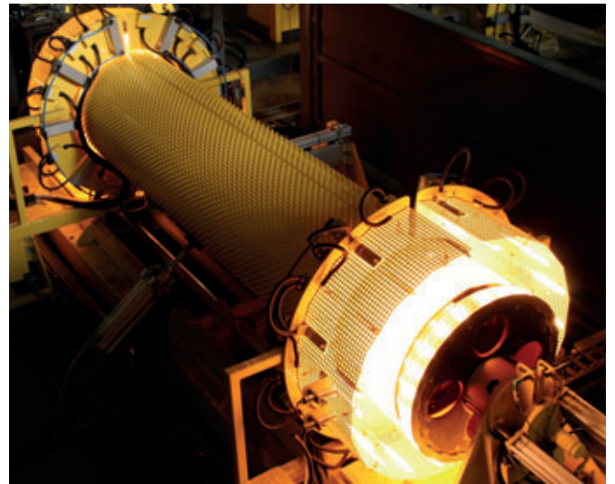
The thermoplastic shaping process to form pipe joints
