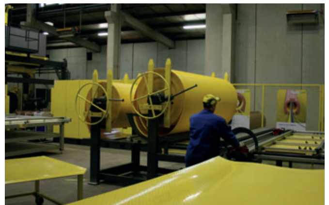
A roll of PE film is cut to length for the production of inliners.
