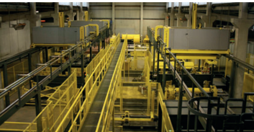
Perfect Pipe manufacturing at Müller in Breisach. The manufacturing process is almost completely automated throughout several stages.
