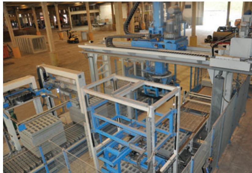
The fully automatic servo cuber takes the products from the production board and forms a block packet on the discharge unit.
