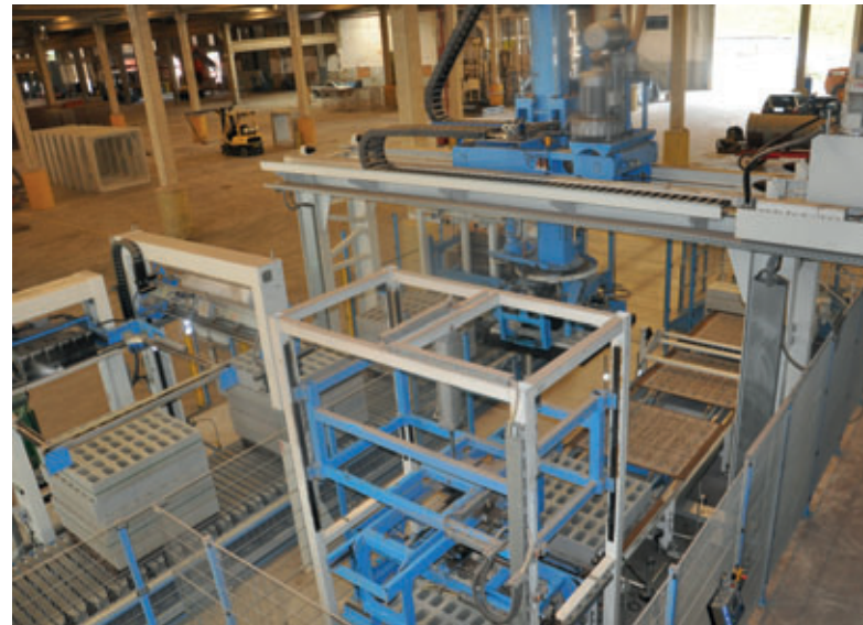
The fully automatic servo cuber takes the products from the production board and forms a block packet on the discharge unit.
