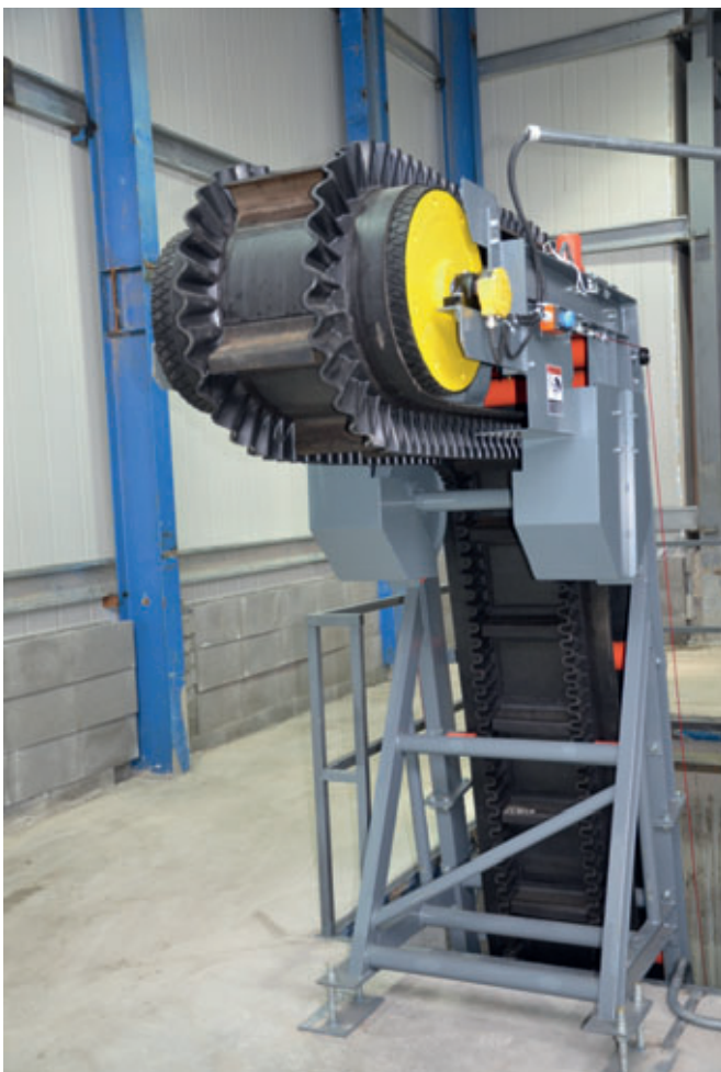
A vertical conveyor belt carries the milled material out of the pit
