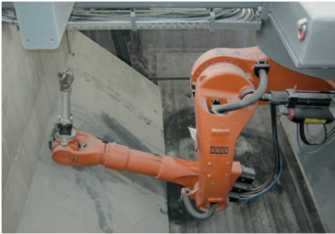
The milling robot works below ground level
