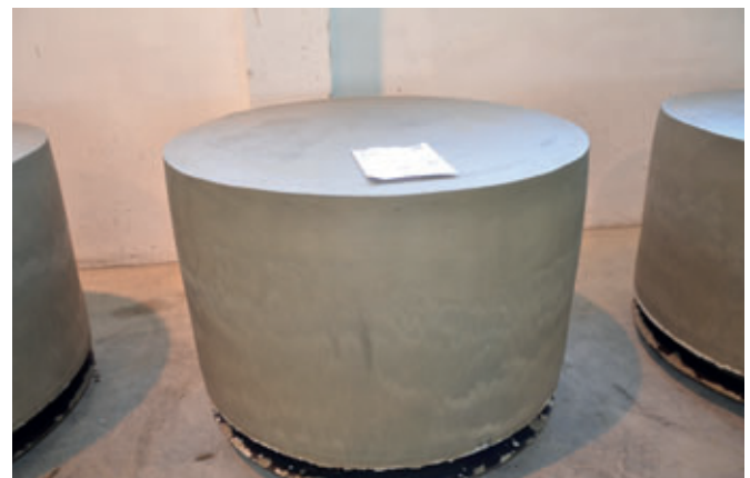
Blanks are stripped of their formwork immediately for milling
