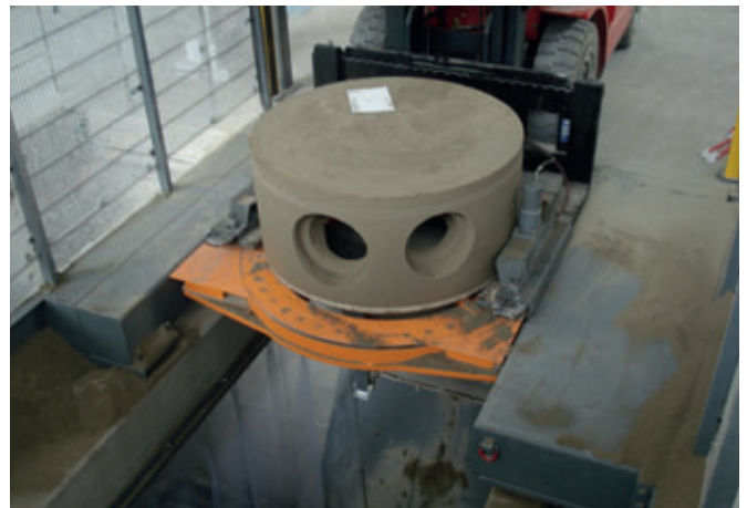
Once milling the manhole base section has been completed, it is transported out of the processing bay
