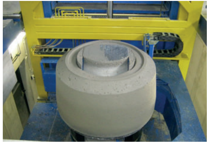
Manufacturing manhole cones on the Tornado
