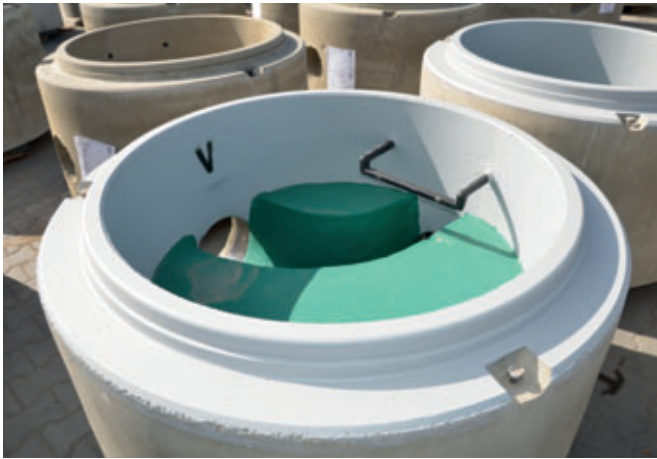
The channel and connections are milled fully automatically; the drill holes for the climbing stirrup are also set in place
