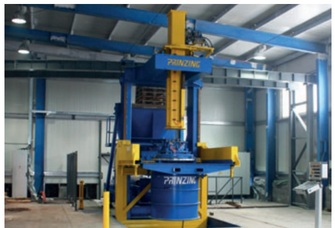
Extremely short retooling times with the Tornado enable different products, such as manhole rings, cones and base blanks, to be produced in one shift
