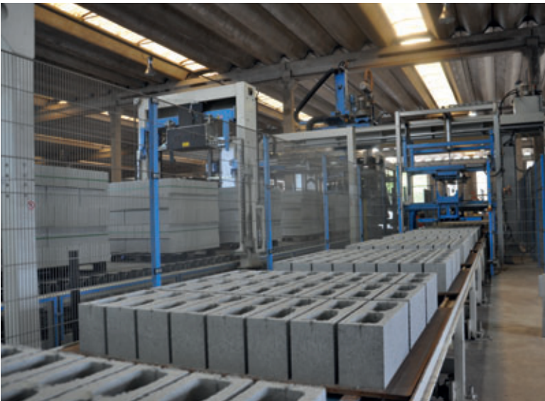
Walking beam conveyor on the dry side
