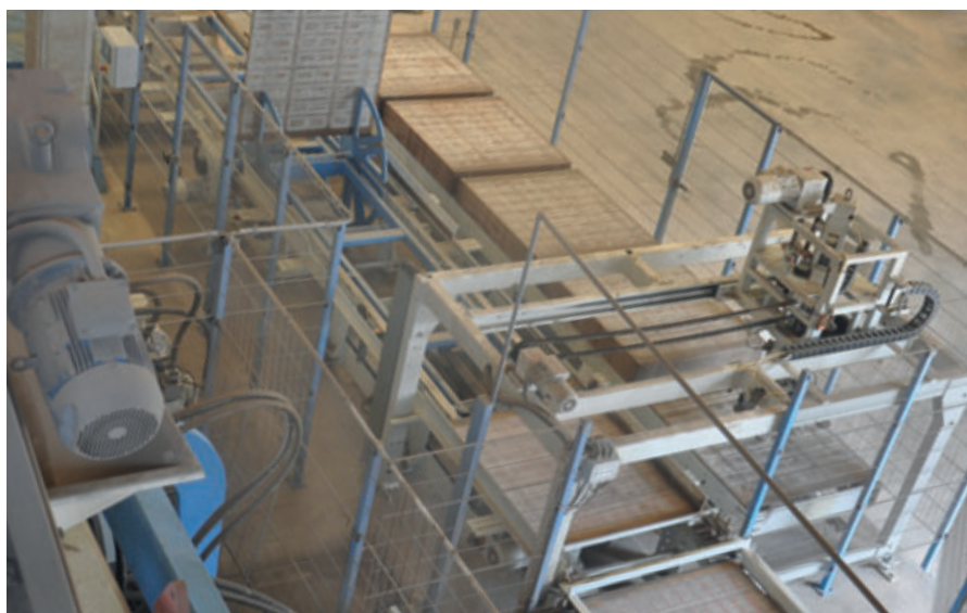
The cleaned boards are turned over and fed to the machine's board silo by a transverse transporter
