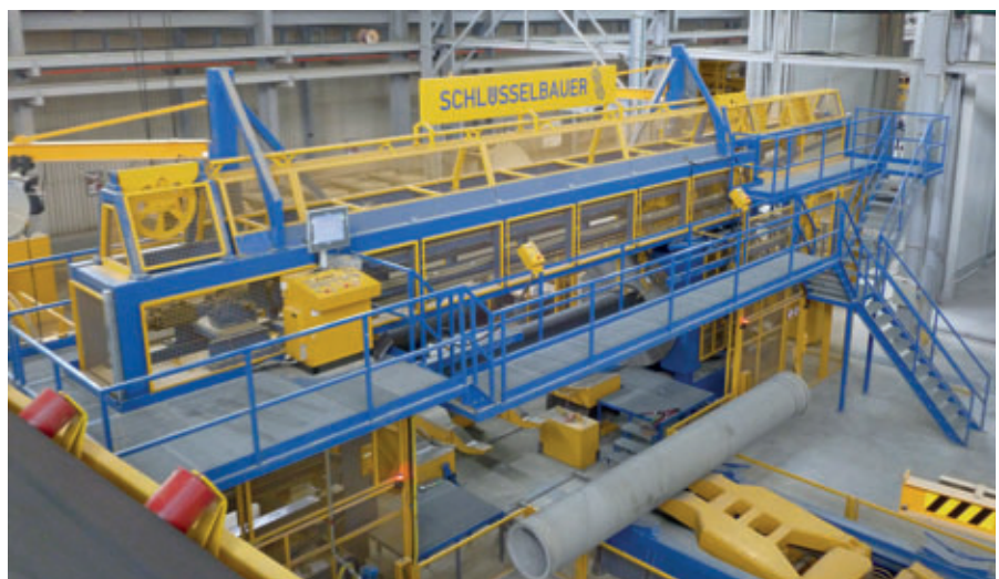
The pre-stressing machine developed by Schlüsselbauer works at a wrapping speed of up to 6 m/s.
