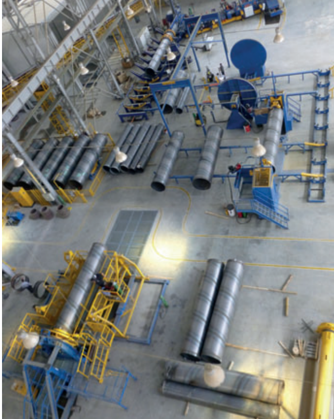
For the manufacture of the sheet steel core used for the impermeability of the concrete pressure pipe, a cylinder is automatically welded and cut to length and tested according to the pipe construction length.
