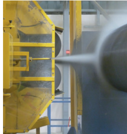
In the final manufacturing step, an external protective layer is applied to the pipe with spun concrete.
