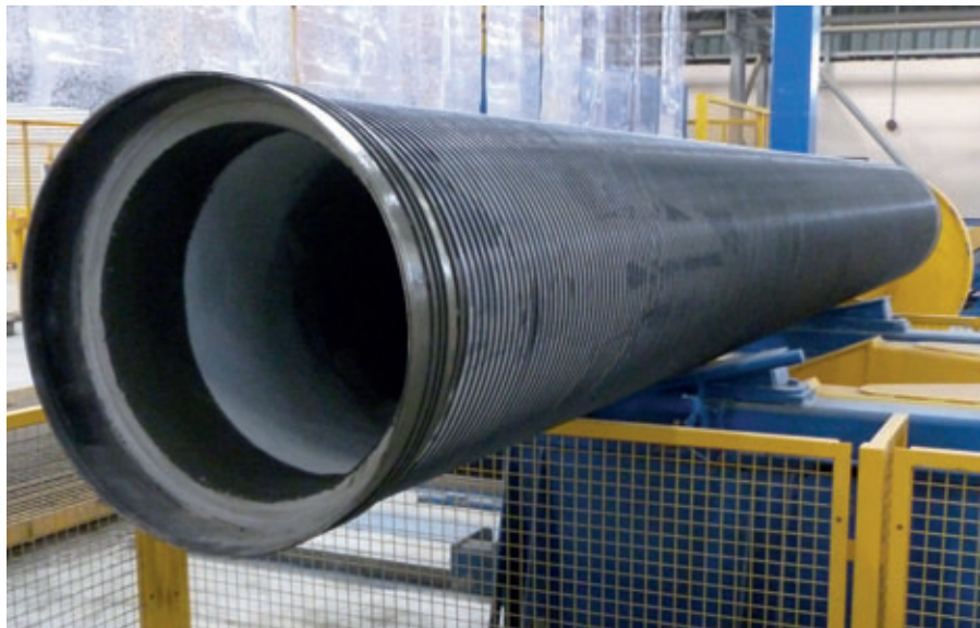
A range of fully automated manipulators move the semi-finished concrete pressure pipes through the production plant. The picture illustrates an insight into the concrete lining of the concrete pressure pipe.
