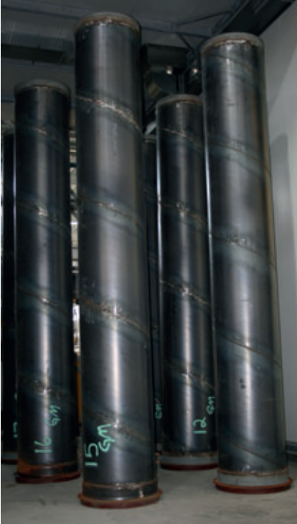
Steel cylinders lined with concrete generally harden in kilns in one day. Completion then follows with application of the pre-tensioned wire and the external coating.
