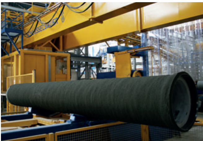
Concrete pressure pipes can be manufactured with different joinings. In the specific project, joints and spigot ends are moulded with steel end rings.
