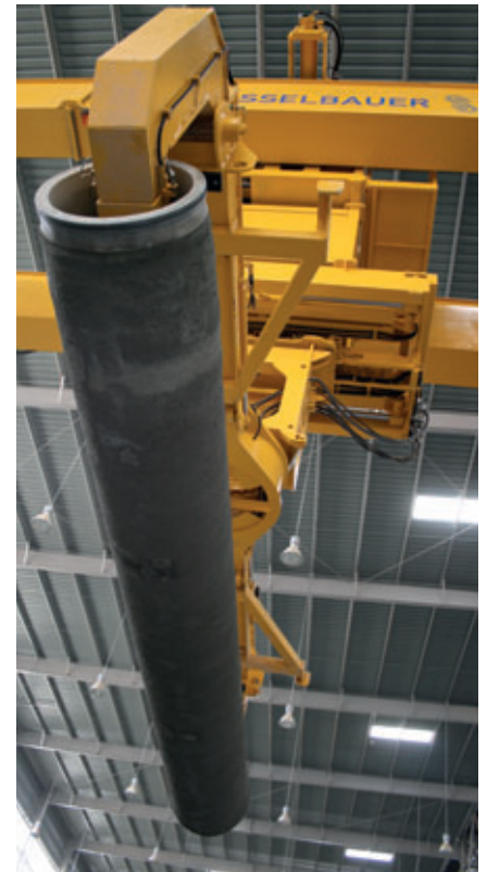
The Schlüsselbauer Transexact automatic crane transports the finished products into the hardening chambers and then to the delivery conveyor belt. It also operates the chamber covers.
