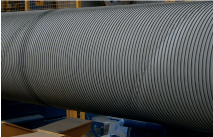
In accordance with the necessary operating pressure of the concrete pressure pipes, wire thickness, pre-stressing and the pitch of the wrapping are determined.
