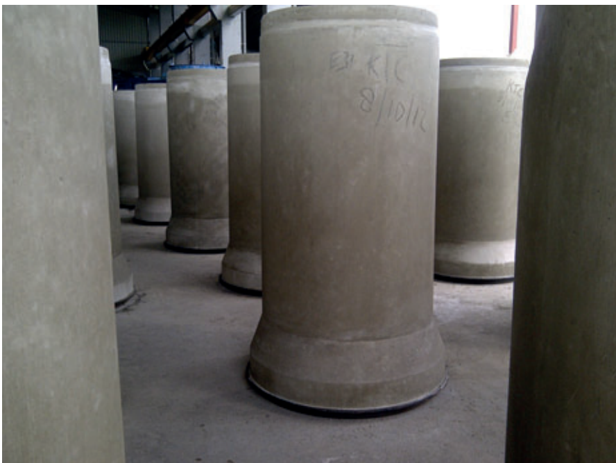
Concrete pipes curing
