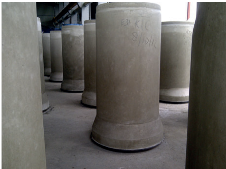
Concrete pipes curing
