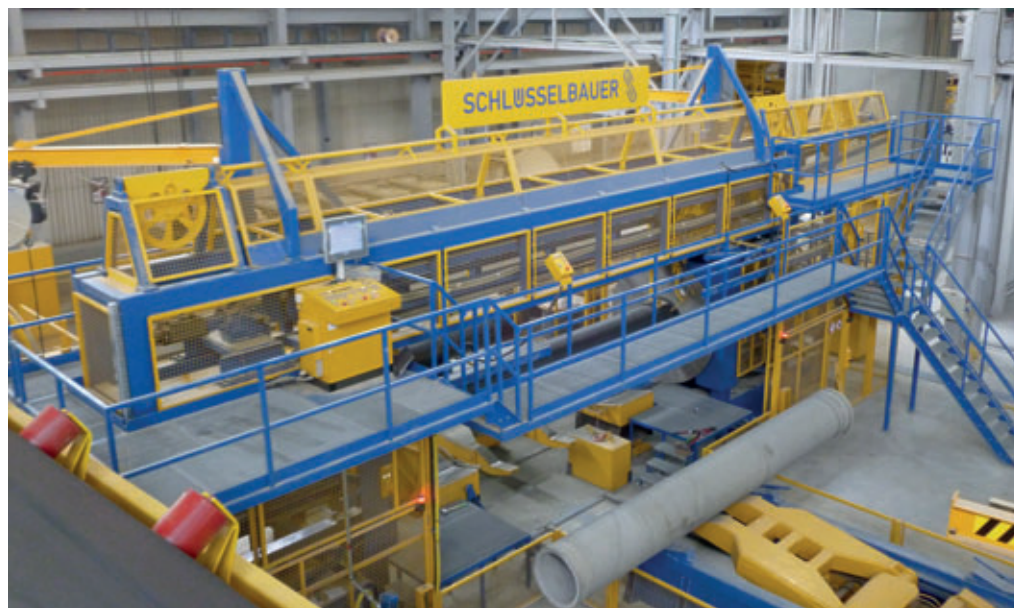
The pre-stressing machine developed by Schlüsselbauer works at a wrapping speed of up to 6 m/s.
