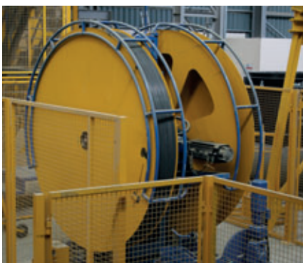
The steel wire required for pre-stressing is also brought to the plant in coils where it is processed with a wrapping speed of up to 6 m/s.
