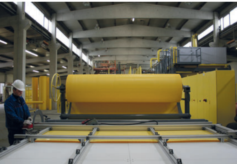
The HDPE inliner tracks are cut to length for a perfect fit according to nominal width and construction length.
