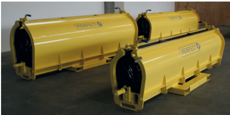
Separate mould equipment is available for the manufacture of link pipes of the nominal widths DN250 to DN600.
