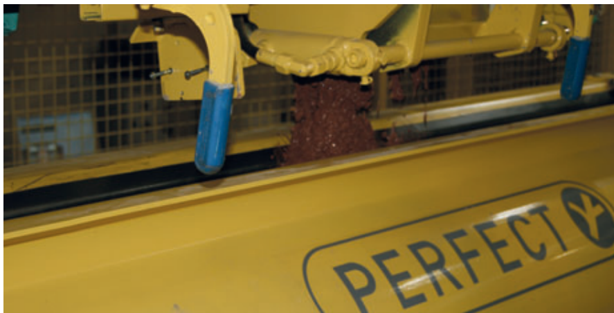
The concreting equipment specifically designed for Perfect Pipe manufacture.
