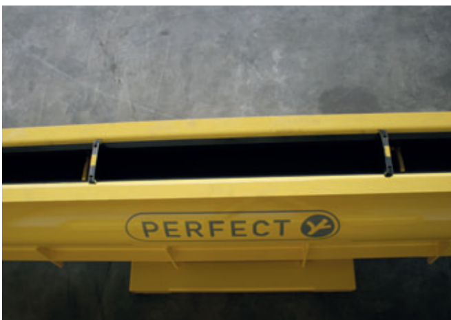
Individually adjustable lateral seals enable individual construction lengths in Perfect Pipe link pipe manufacture.
