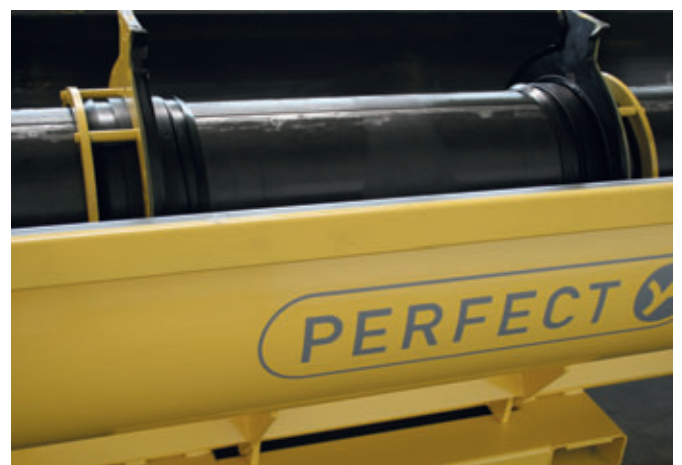
View of a link pipe mould with freely adjustable lateral seals.
