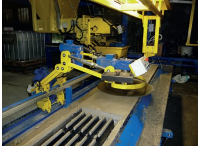
The optional trowelling device can also run in automatic mode
