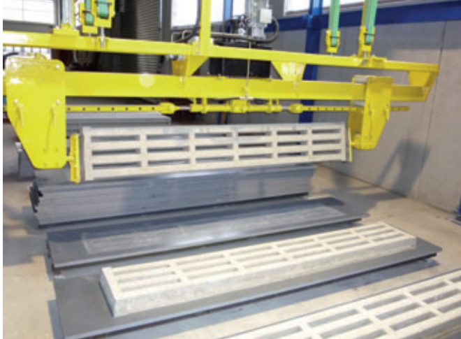
L-3 Product lifting unit with hydraulic clamp
