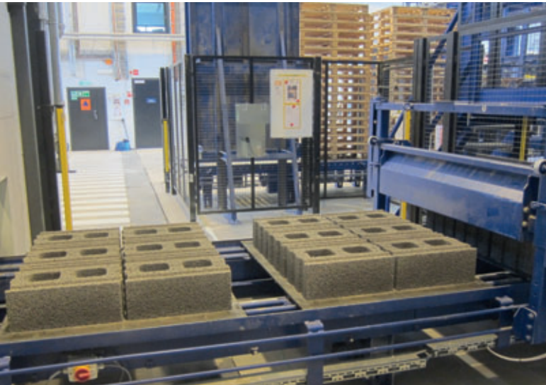
Hardened concrete blocks on the dry side
