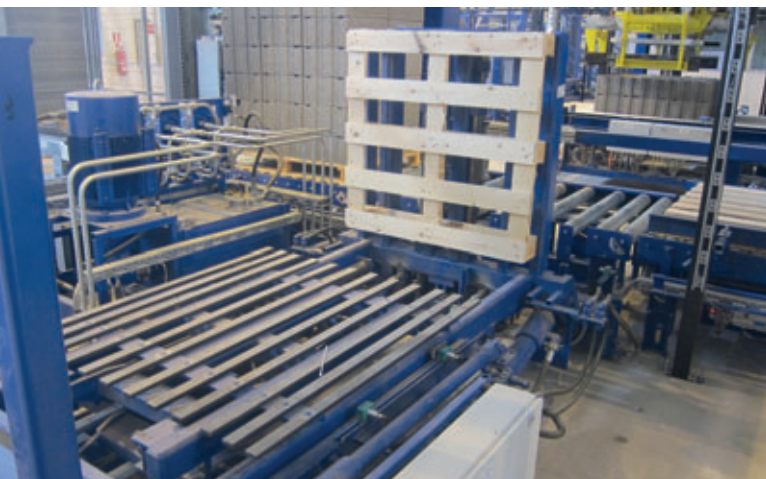
Block packets can be prepared ‘lying down’ with the tilting table.
