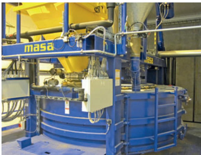
PH 3000/4500 horizontal compulsory mixer from Masa
