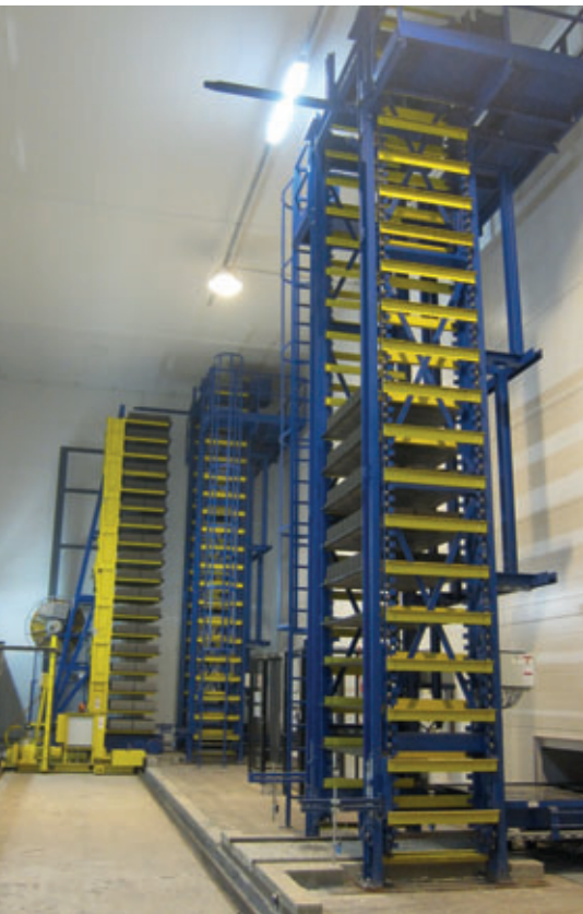
Transfer of hardened concrete goods to the lowerator on the dry side
