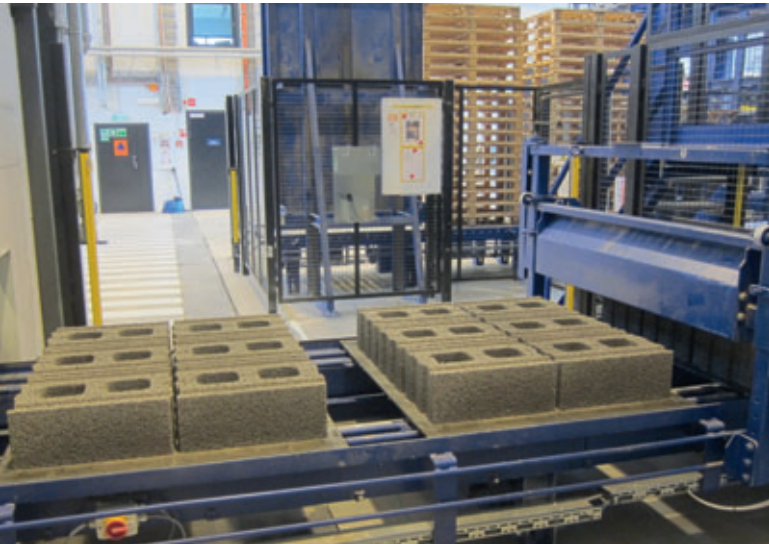
Hardened concrete blocks on the dry side
