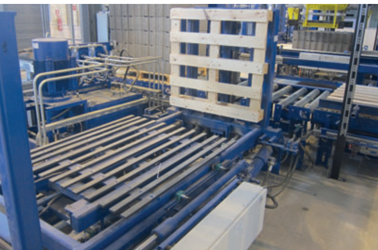
Block packets can be prepared 'lying down' with the tilting table.
