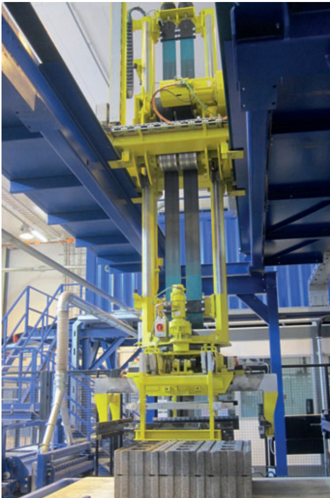
The rotary suspended gripping and clamping device with electrically-driven four-sided clamp
