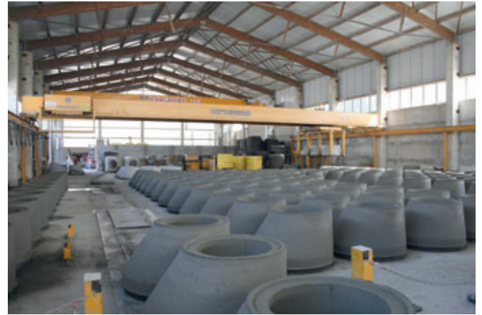
The new Perfect manhole base manufacture is housed in the rear section of this hall, where precast manhole components have been produced with a Schlüsselbauer Exact plant for years.
