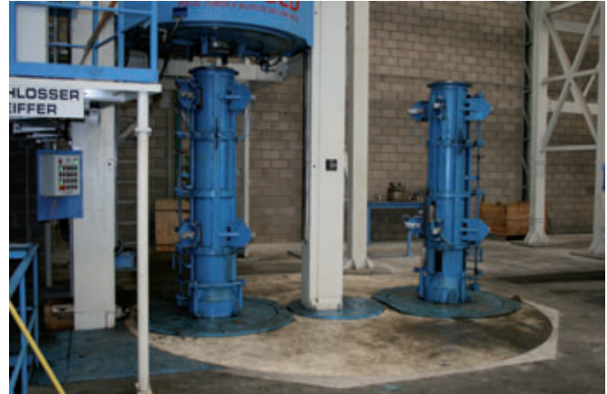
The turn table hands over a mold with a finished pipe to the forklift while at the same time supplying the machine with an empty mold for the production of the next pipe.
