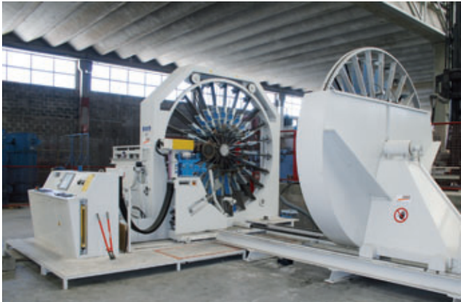
The MBK cage welding machine is producing all cages for round pipe produced at Tecmold
