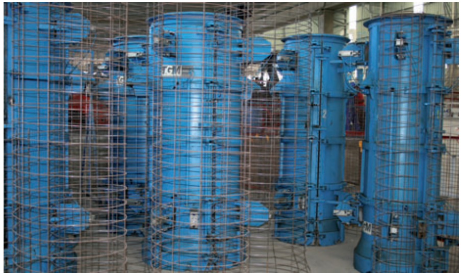
The molds for the pipes and box culverts were supplied by TGM
