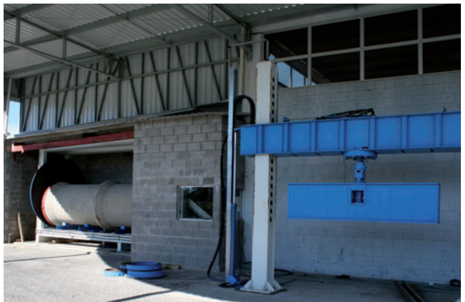
Tecmold is testing tensile splitting force capacity and density of the pipe according to Brazilian NBR standards
