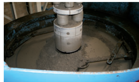
The molds are automatically filled with the correct amount of concrete, while the rising pressing unit is forming the pipe from the inside
