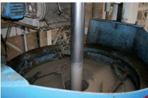
The molds are automatically filled with the correct amount of concrete, while the rising pressing unit is forming the pipe from the inside
