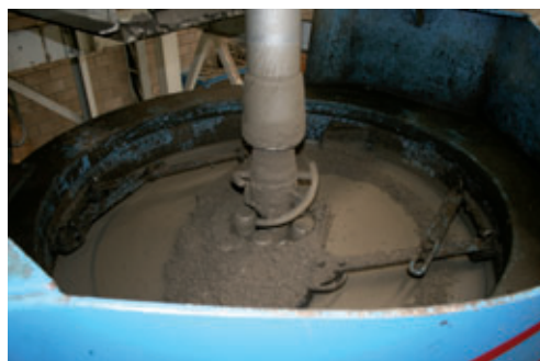
The molds are automatically filled with the correct amount of concrete, while the rising pressing unit is forming the pipe from the inside
