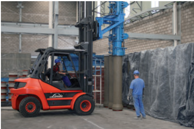
Finished pipe are transported by forklifter to the curing area where they are demolded and covered with foil for 24 hours
