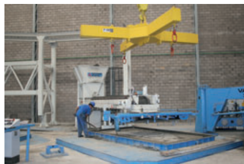
The Schlosser-Pfeiffer Variant is a versatile machine to produce large pipe and box culverts
