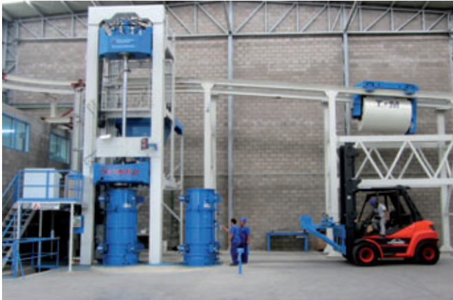
The radial press RP 1225-4 is producing pipe from 300-1500mm diameter
