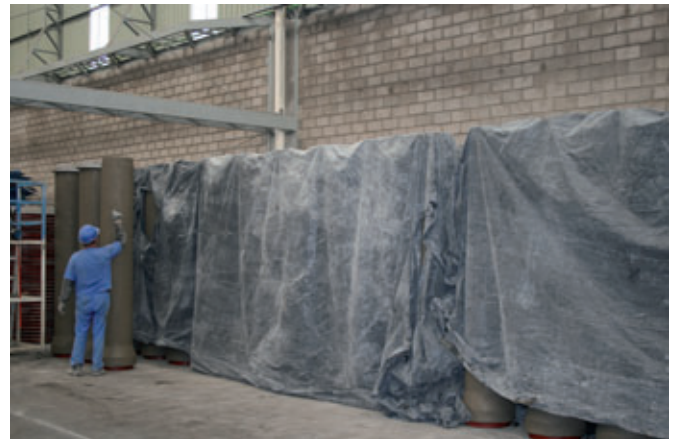
Finished pipe are transported by forklifter to the curing area where they are demolded and covered with foil for 24 hours
