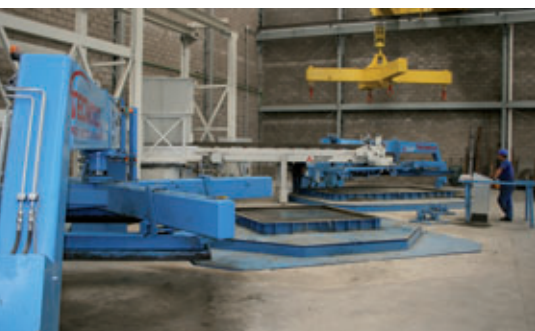
The Schlosser-Pfeiffer Variant is a versatile machine to produce large pipe and box culverts
