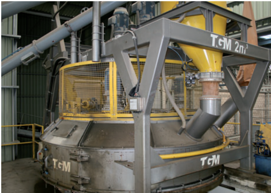
The 2m 3 mixer compulsory mixer, similar to the Schlosser-Pfeiffer SM mixer, is particularly suitable for the production of dry concrete
