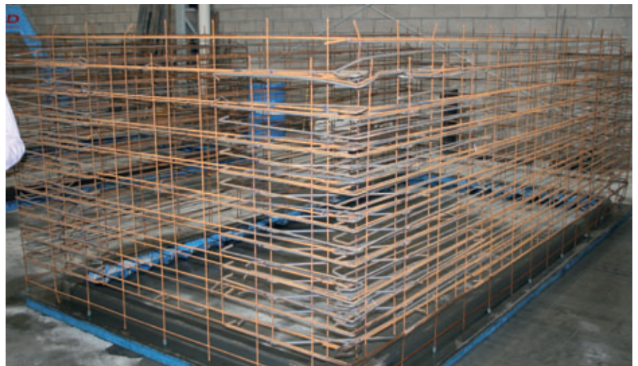
The reinforcement cages for large diameter pipe and box culverts are currently produced manually very efficiently. With 8 workers, it takes less than 1 hour to produce the cage for a 4.000x2.000mm box culvert.
