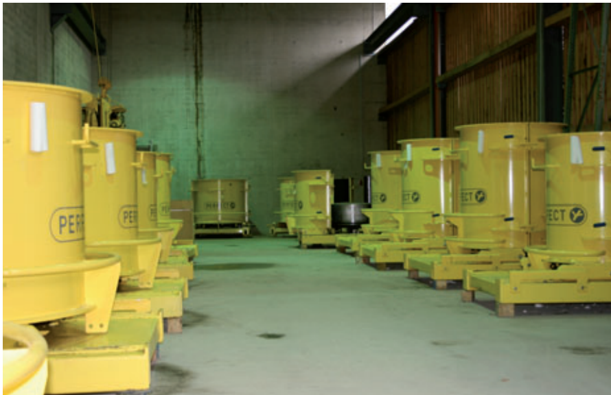
In total, 16 moulds are available for filling with self-compacting concrete in the start phase at the Rhomberg concrete plant.
