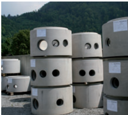
Numerous projects are accomplished with custom-made manhole subcomponents approximately two months after commissioning the Perfect manufacturing system.
