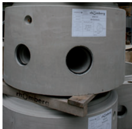
Regardless of the wall thicknesses of the manhole subcomponent, transport anchors are laterally encased into the wall or in the contact area for manhole rings.
