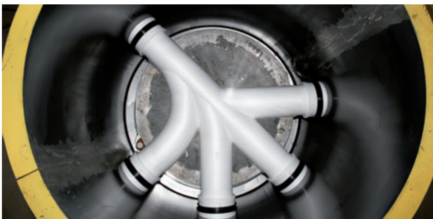
Several intakes are also combined in manhole bases < DN1000. – This picture shows a prepared mould for a DN 800 manhole subcomponent.
