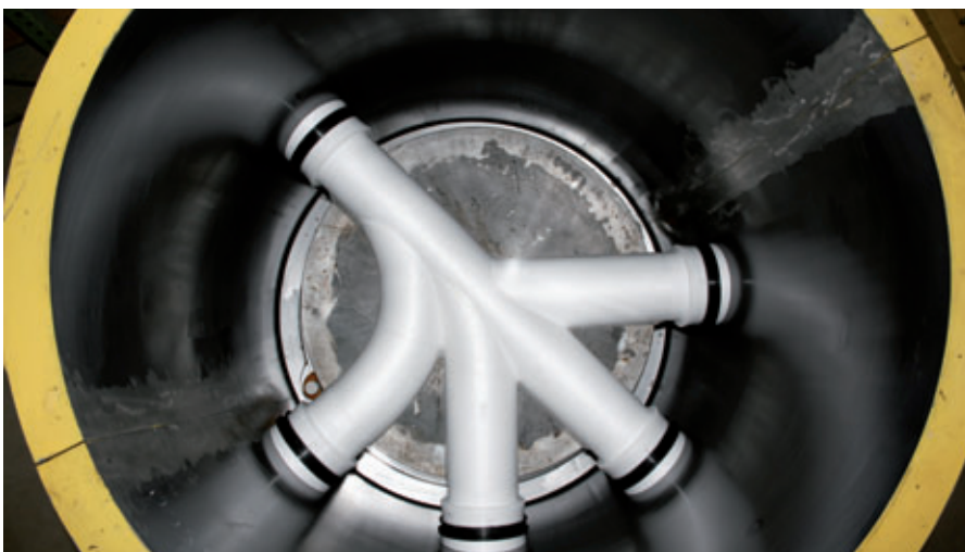
Several intakes are also combined in manhole bases < DN1000. – This picture shows a prepared mould for a DN 800 manhole subcomponent.
