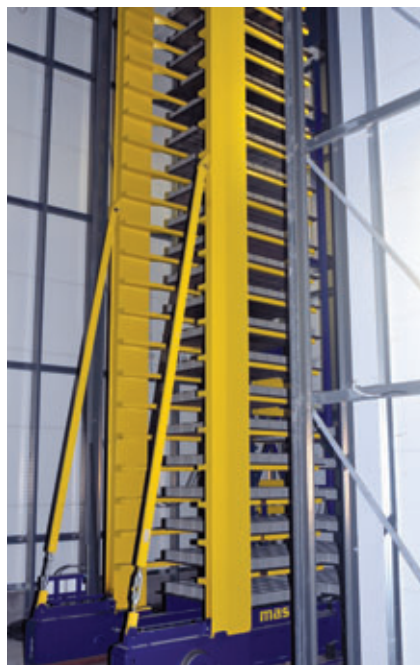
Pre-lift in the form of a mobile buffer between the transfer table and lowerator
