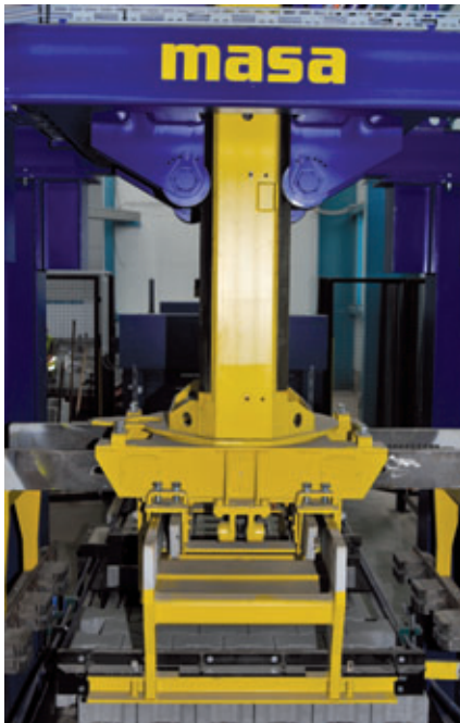
Detailed view of a four-sided centring unit with servo drives
