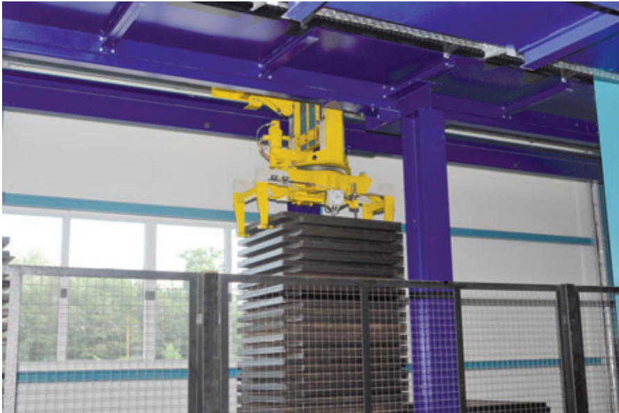
Pallet packet gripper for putting the production pallets into and taking them out of the pallet store
