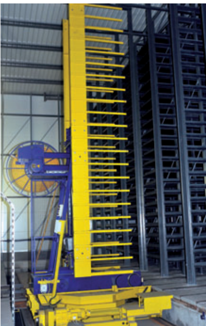
Transfer table and rack system
