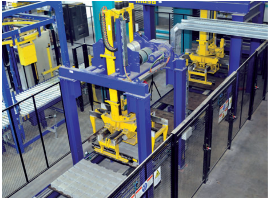
Return transport with four-sided centring and packet assembly
