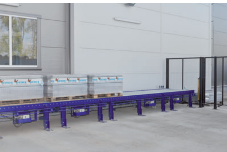
Packet transport to removal by fork lift truck
