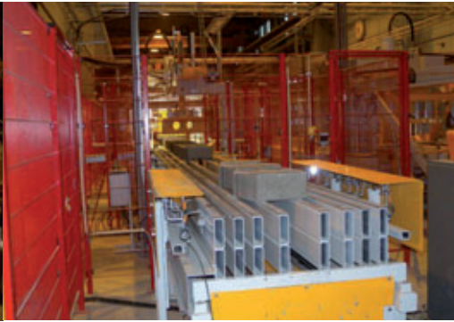
Formatted products before removal by robot
