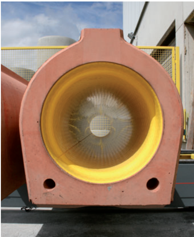
The base pipe geometry facilitates construction site use and accuracy of the pipeline. The flat bottom surface also facilitates handling for storage and transport.
