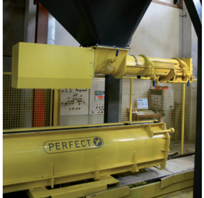
The concrete encasing station is continually supplied with SCC from the mixing plant via a transfer hopper.
