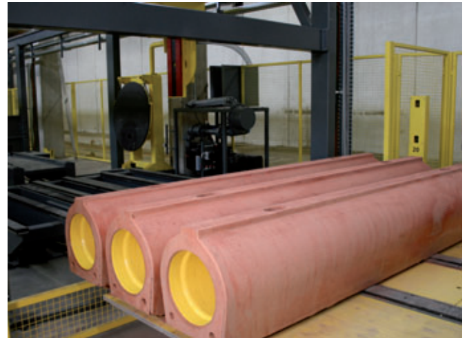
The demoulded products are placed in groups on the outfeed belt according to the nominal width after an in-line vacuum test and conveyed out of the hall for storage or delivery.
