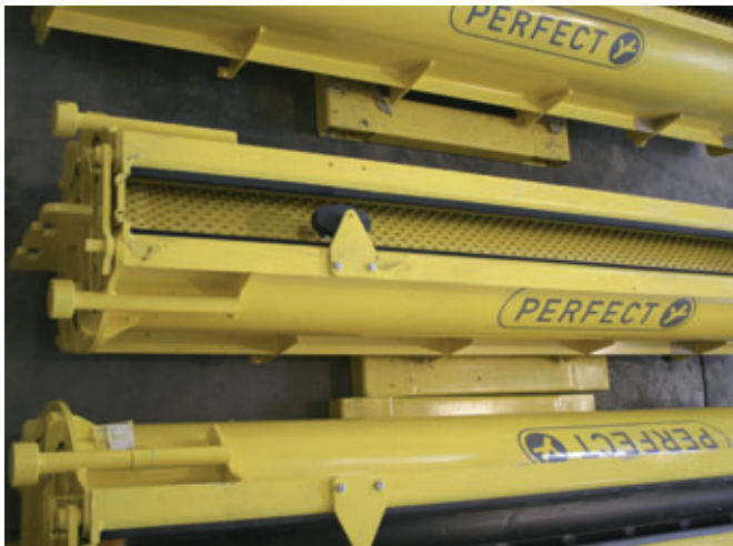
The shapes designed for horizontal manufacture are available with or without a liner for the concrete encasing process which is also automated.
