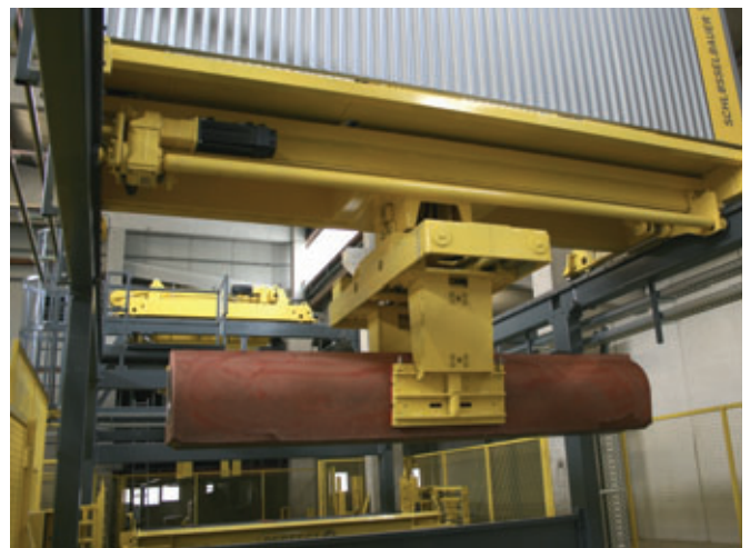
An additional robot accepts the product after automatic opening of the moulds.
