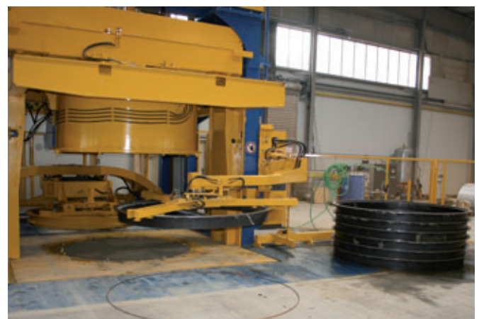
One-man operation of the entire production plant by automated processes, only the insertion of the reinforcement ring is manual.
