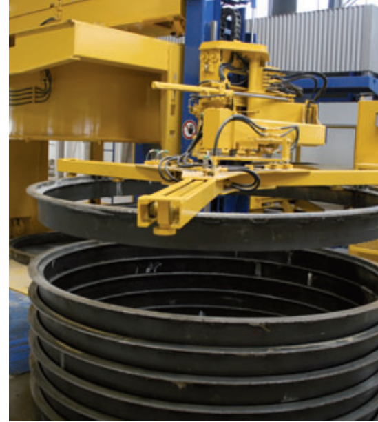
The automatic pallet feeding device is a crucial element in the one-man operation of this plant.
