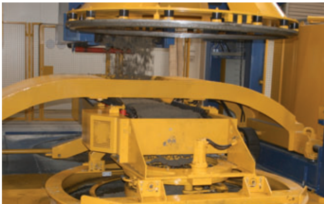
The entire concrete supply of the Magic2500 was newly constructed with a view to rapidly inserting concrete into the machine
