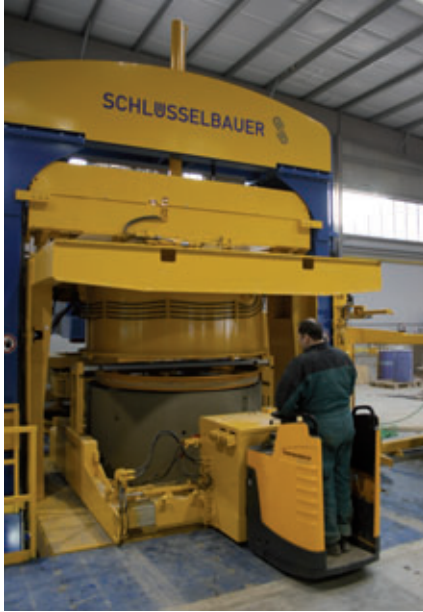
An electrical truck with a retaining ring manipulator used for removal of the products
