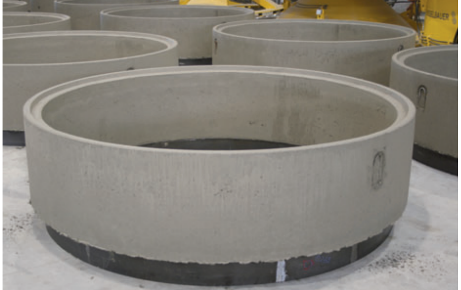
DN1500 manhole rings in the setting area
