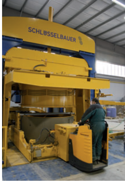
The support ring manipulator permits the operator to effortlessly place the support rings on the new product without being assisted by a second worker
