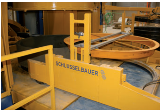
An innovation in the manipulation of support rings – a manipulator undertakes the work-intensive process of fitting support rings
