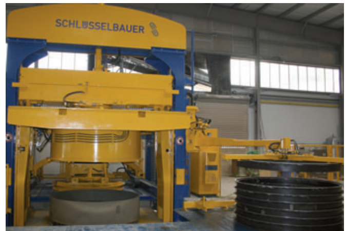
The Magic2500 production plant for the manufacture of precast components with an external diameter of up to 2700 mm
