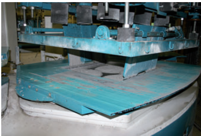
Figure 2: Hose-type dosing unit for filling the facing concrete
