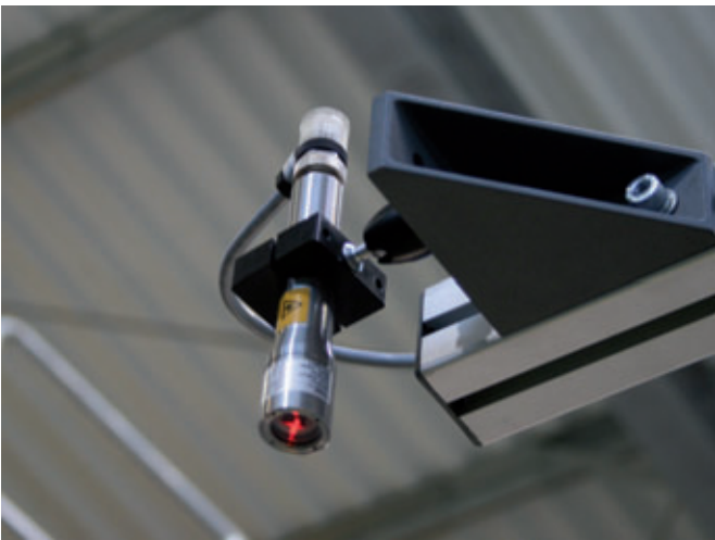
In-line-quality check by laser
