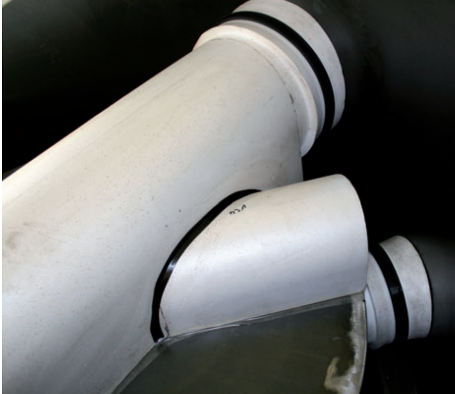
Negative EPS channel positioned in the steel mould with a gradation typically for the region
