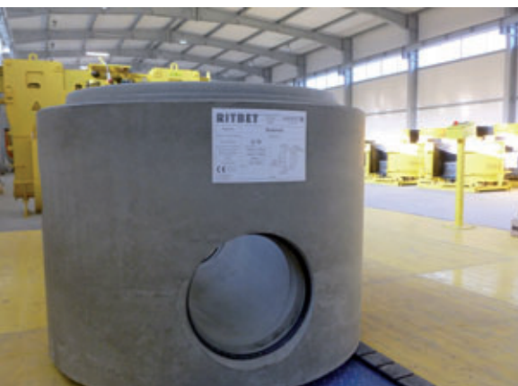
Labelled with an easy to read data sheet Perfect monobases are leaving the production hall
