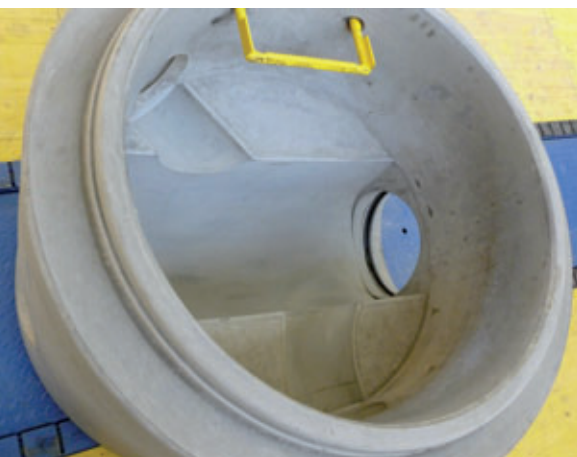
Finished manhole base with mouted stepung
