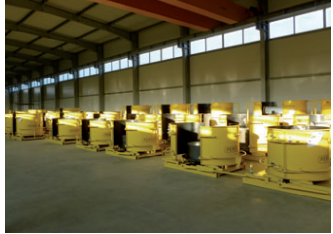
A set of various Perfect moulds allows production of up to 33 manhole bases per shift with three different diameters, an extra mould was set in for larger products
