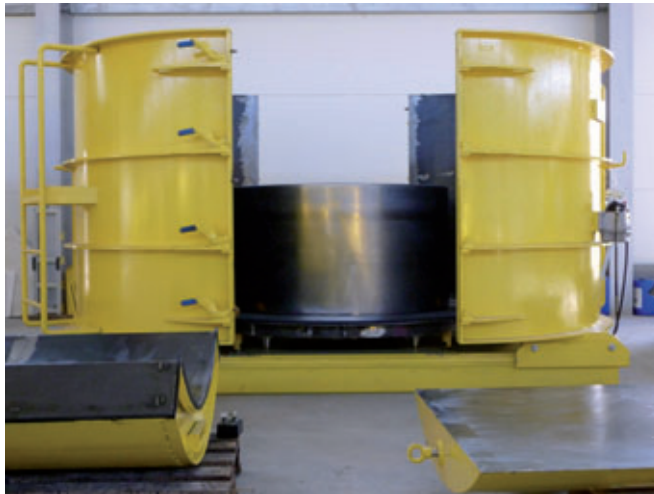
Large Perfect mould with partial wall thickness reduction elements
