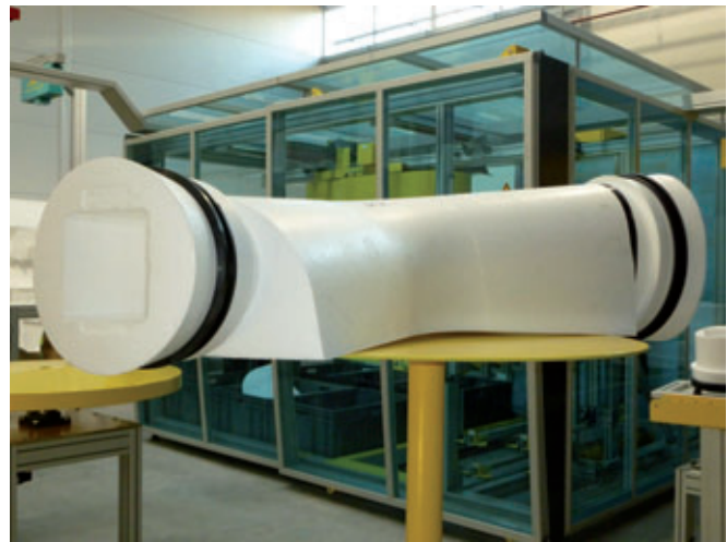
Gaskets mounted on the holeformer mean dense pipe connections in the precast product
