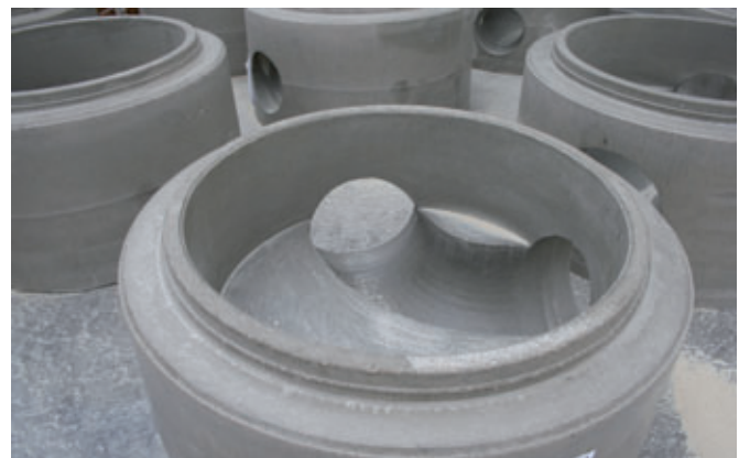
The concrete manhole bases milled with the Primuss method were very popular right from the start
