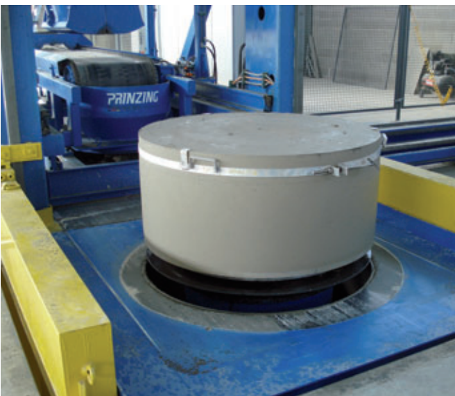
Raw manhole base blank after demoulding. After a short hardening time the blank can be taken to the milling station.
