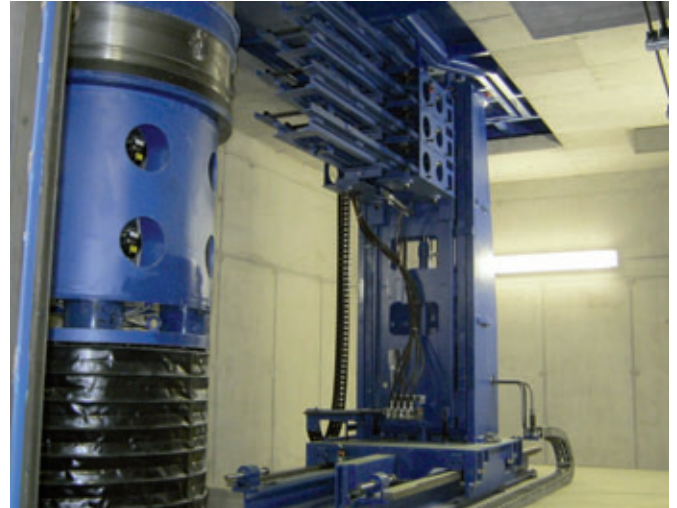
Automatic step magazine for manhole ring and cone production
