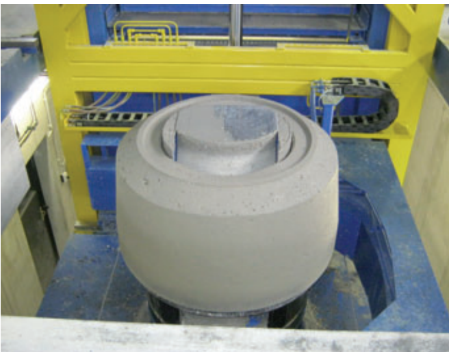
Manhole cone during demoulding in the Tornado machine. Dolomit uses the Tornado to produce the full range of manhole products: cones, rings and bases
