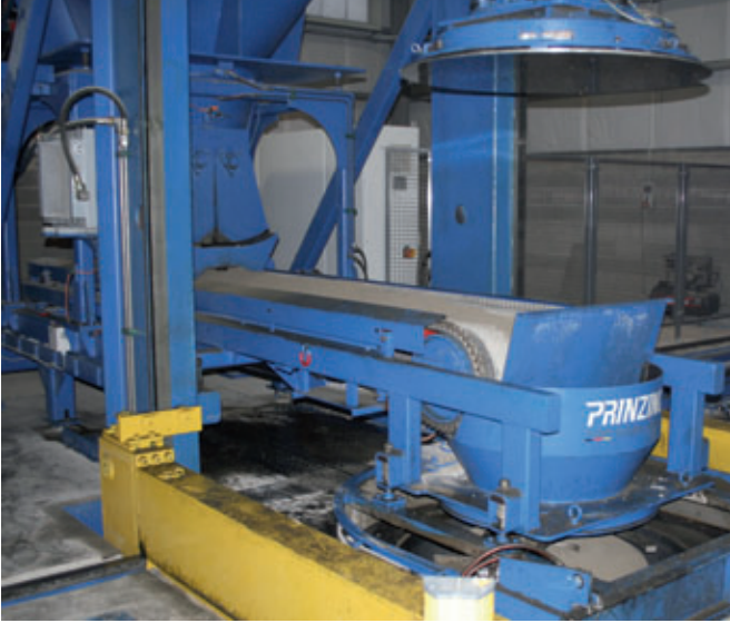
Dosing shutters below the concrete reservoir ensure optimised mould filling
