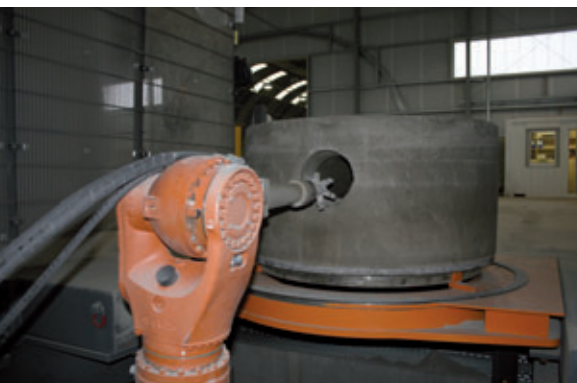
Once a connection has been milled, the robot arm moves back and the manhole is automatically turned to the next milling position.
