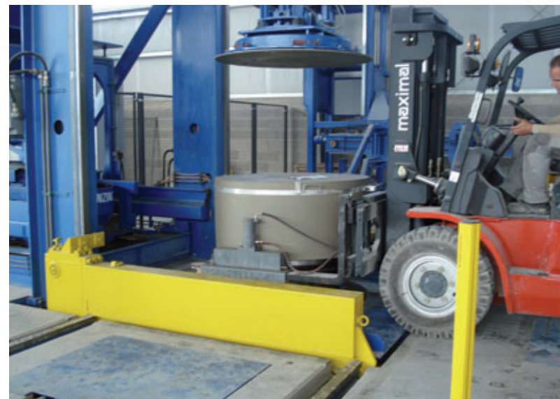
Removal of base blank from the Tornado machine
