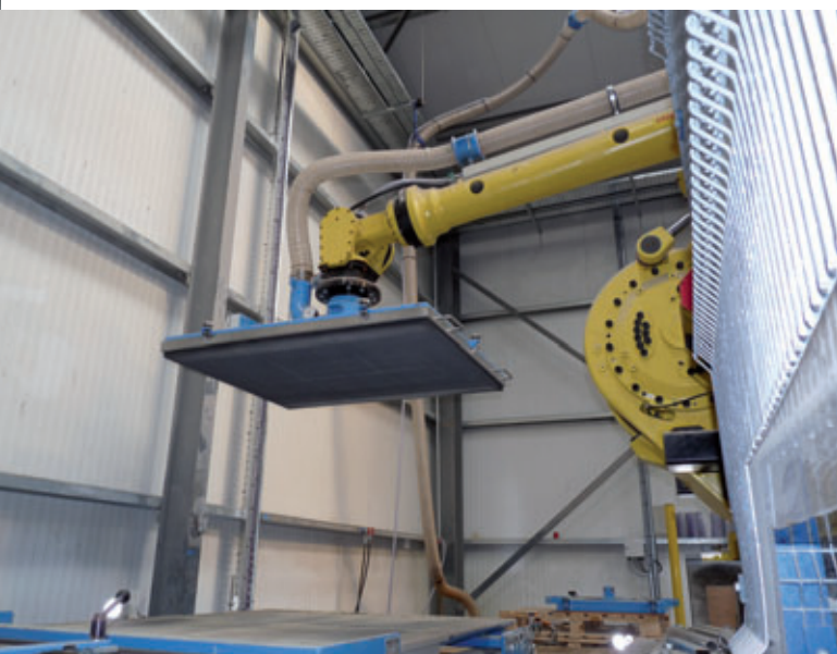
Upon flat and on edge packing a vacuum suction plate mounted at the robot wrist is used.
