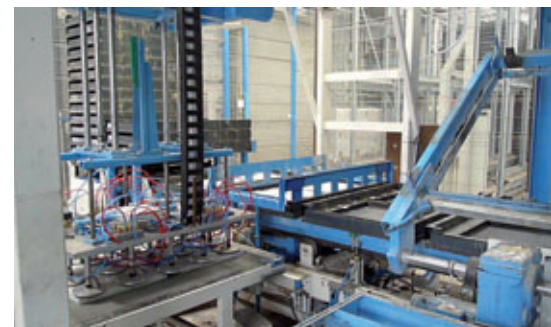
Demoulded products deposited on belt
