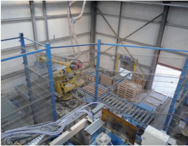
Fanuc robot takes off the products individually after quality control
