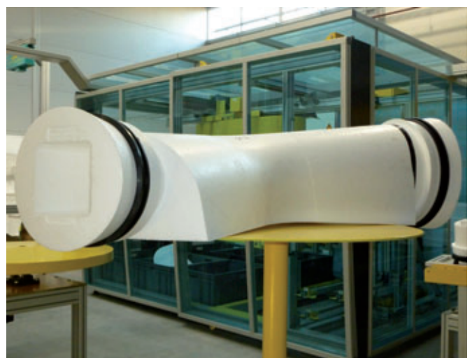
Gaskets mounted on the holeformer mean dense pipe connections in the precast product
