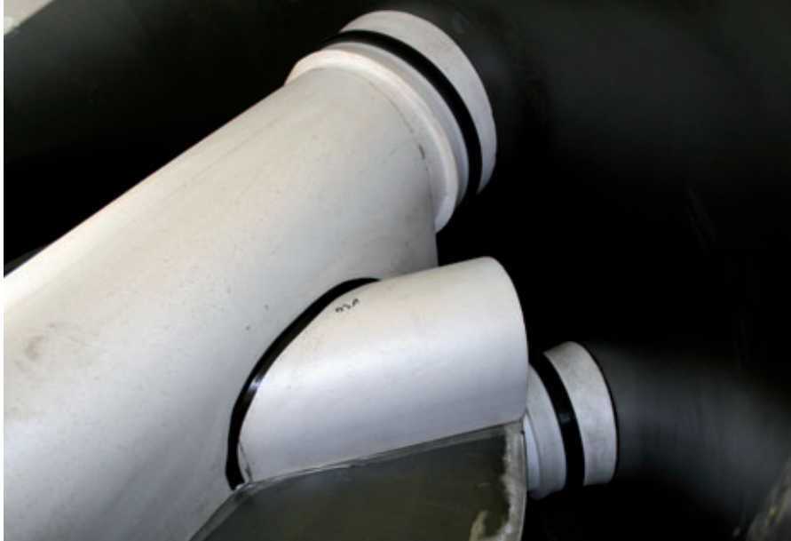
Negative EPS channel positioned in the steel mould with a gradation typically for the region
