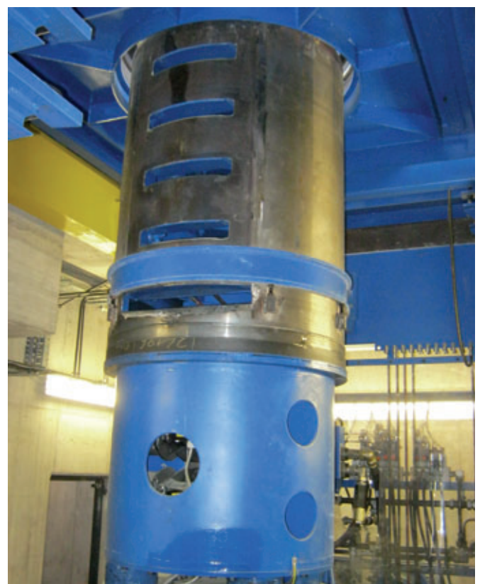
Manhole mould core for direct integration of manhole steps
