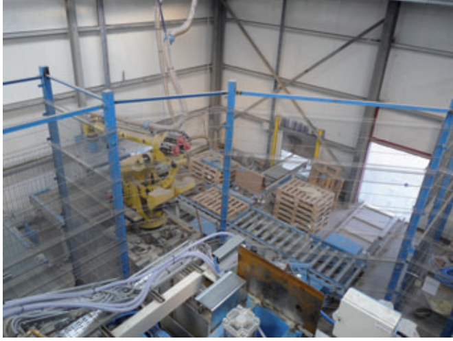
Fanuc robot takes off the products individually after quality control
